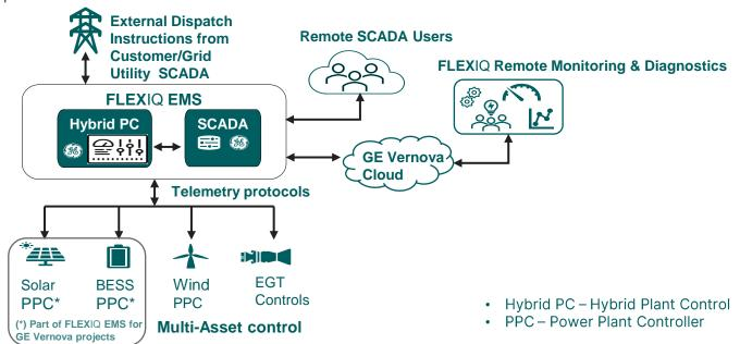
FLEXIO EMS provides a unified and dynamic control & software platform to enable optimized system performance to meet individual Solar and Storage site requirements, allowing information to be shared between plant assets and enterprise applications.
