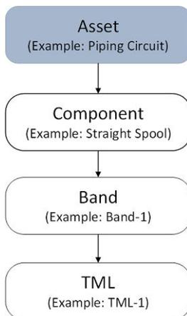
A piping asset can be a piping circuit, and a piping component can be a straight spool or an elbow. A piping component can consist of several bands positioned at various locations on its surface. A band is a path along the circumference or length of a piping component that contains equally spaced TMLs. These TMLs are located at specific positions on the band.
