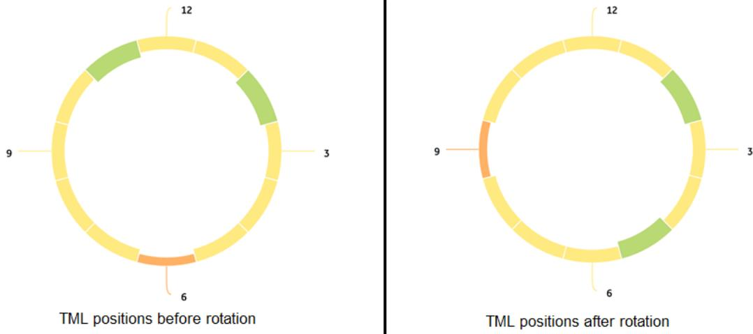
After a spool is rotated, the corrosion analysis for each TML within the bands is re-calculated based on the corrosion rate at the new position. This results in an updated remaining life for the component.
