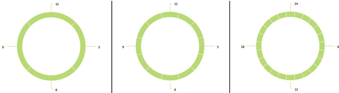
For example, in a piping component, if each band contains 4 TMLs, you can select a configuration of 4 positions. In this configuration, 4 equally spaced reference points (that is 3, 6, 9, and 12) are available along which the component can be rotated. The reference point for rotation is the Top Center. In this example, position 12 is the Top Center.
