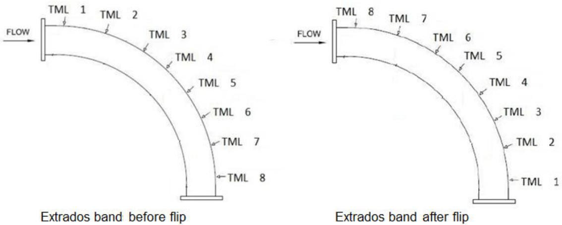
After an elbow is flipped, the corrosion analysis for each TML within the bands is re-calculated based on the corrosion rate at the new position. This results in an updated remaining life for the component.
