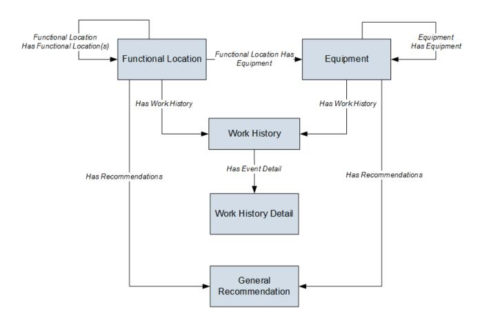
**Note:** In the diagram, boxes represent entity families and arrows represent relationship families that are configured in the baseline database. You can determine the direction of each relationship definition from the direction of the arrow head: the box from which the arrow originates is the predecessor, and the box to which the arrow head points is the successor.
