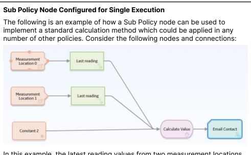
In this example, the latest reading values from two measurement locations and a constant value are passed into a sub policy, which calculates a value to be used in the Email node. The **Properties** window for the Sub Policy node is shown in the following image:
