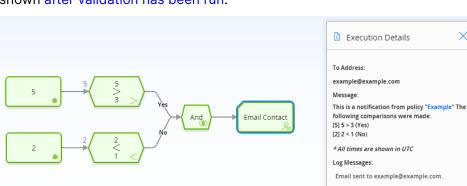
In this example, you can see that each node executed successfully. The logical result of the And node is yes because all incoming logic paths result in a value of true passed to the And node (that is, the logical result of each preceding condition node matches the logic path of the corresponding connection). Therefore, policy execution continues past the And node.
