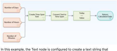
In this example, the Text node is configured to create a text string that indicates a time span, using the values represented by the Point Value nodes. Because the Subtract node cannot perform any calculation on a text string, the Convert Type node converts the string to a value of the Time Span data type. The converted time span value is then used in the Subtract node to calculate the required date.
