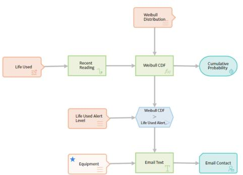
The threshold percentage of life used for the equipment is stored as a Technical Characteristic. The life data of the equipment (for example, hours for turbine, starts for crane, take-offs for aircraft, tonnes moved for mining equipment), is stored as Measurement Location readings.
