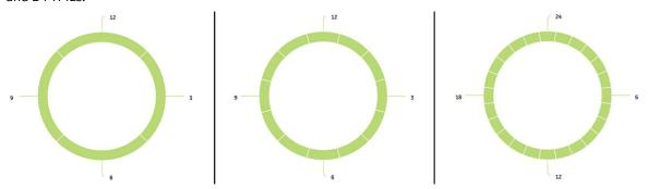
For example, in a piping component, if each band contains 4 TMLs, you can select a configuration of 4 positions. In this configuration, 4 equally spaced reference points (that is 3, 6, 9, and 12) are available along which the component can be rotated. The reference point for rotation is the Top Center. In this example, position 12 is the Top Center.
