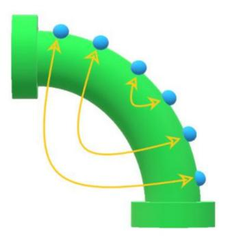
The arrows show the movement of TMLs on the band after a flip. Each TML exchanges position with its mirrored TML within the band. The following image illustrates the positions of TMLs in an extrados band before and after flipping the elbow.
