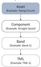
A piping asset can be a piping circuit, and a piping component can be a straight spool or an elbow. A piping component can consist of several bands positioned at various locations on its surface. A band is a path along the circumference or length of a piping component that contains equally spaced TMLs. These TMLs are located at specific positions on the band.
