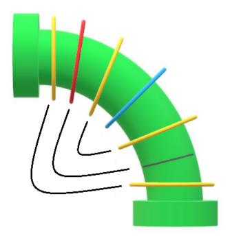
The bands colored yellow are mirrored bands, and the band colored blue is the center band. The band colored red is an odd band. When the elbow is flipped, the TMLs on the odd band move to a different location on the elbow, where a band did not previously exist.
