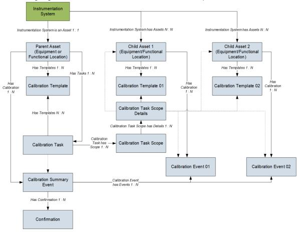
**Note:** In the diagram, boxes represent entity families and arrows represent relationship families that are configured in the baseline database. You can determine the direction of each relationship definition from the direction of the arrowhead: the box from which the arrow originates is the predecessor, and the box to which the arrowhead points is the successor.
