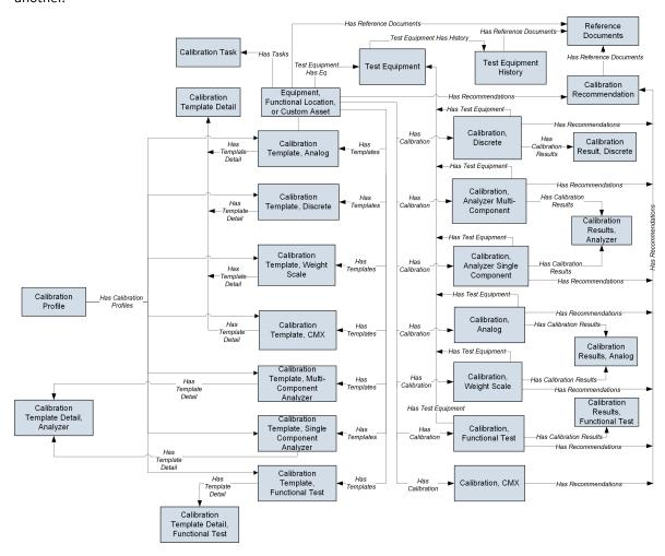
The following diagram shows how the families used in device mapping in Calibration Management are related to one another.
