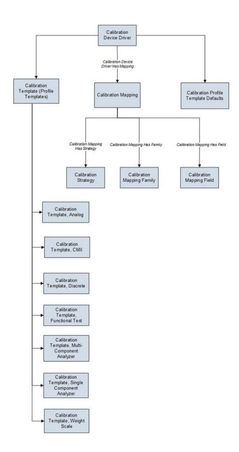
**Note:** In the diagram, boxes represent entity families and arrows represent relationship families that are configured in the baseline database. You can determine the direction of the each relationship definition from the direction of the arrow head: the box from which the arrow originates is the predecessor, and the box to which the arrow head points is the successor.
