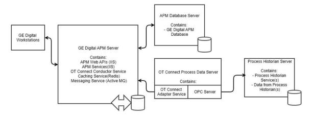
The Conductor requires access to the APM Datasource(s), so it should be installed on the APM Server with the other services.
