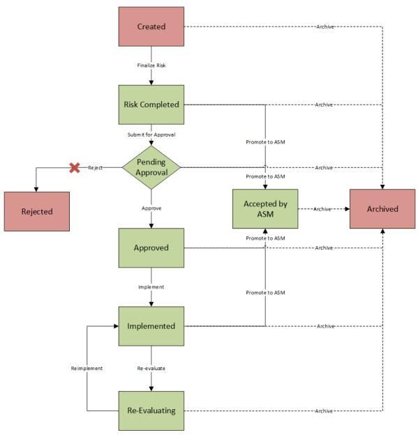
Notice that the some of the states are highlighted in Green. When an RBI Criticality Analysis is set to any of these states, the analysis is active. When an RBI Criticality Analysis is set to any of the states highlighted in Red, the analysis is inactive.
