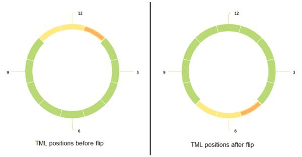
The following table illustrates the band positions for center and mirrored bands before and after a flip for an elbow with 12 band positions.
