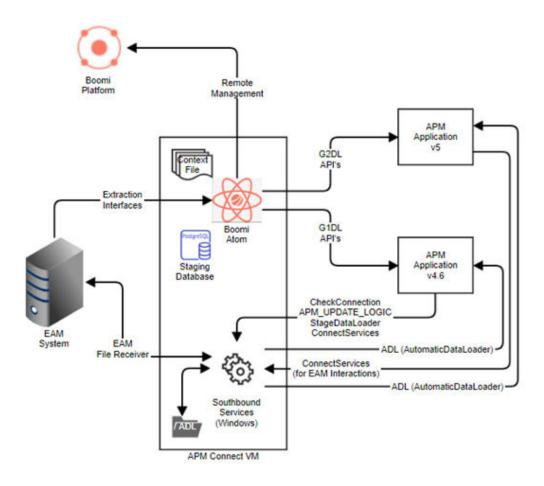
In an on-premise architecture, the Boomi Atom runs on the APM Connect server to facilitate extractions from the EAM system. This functionality is supported by configurations specified in the Context File and
