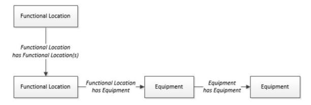
The Functional Location can be linked to a parent Functional Location using the relationship Functional Location Has Functional Location(s).
