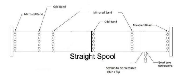
The following diagram illustrates the bands that can exist on a straight spool.
