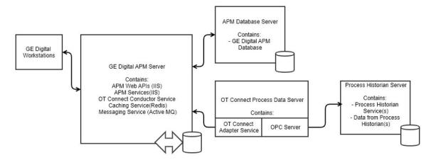
The Conductor requires access to the GE Digital APM Datasource(s), so it should be installed on the GE Digital APM Server with the other services.
