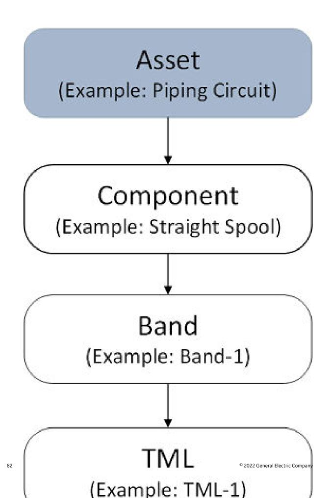
A piping asset can be a piping circuit, and a piping component can be a straight spool or an elbow. A piping component can consist of several bands positioned at various locations on its surface. A band is a path along the circumference or length of a piping component that contains equally spaced TMLs. These TMLs are located at specific positions on the band.
