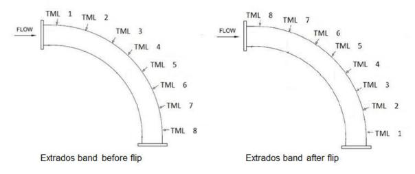
After an elbow is flipped, the corrosion analysis for each TML within the bands is re-calculated based on the corrosion rate at the new position. This results in an updated remaining life for the component.
