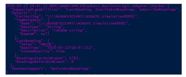
This report shows that we have successfully connected to the configured OPC-HDA server, and received both metadata and Readings for the provided TestTag.
