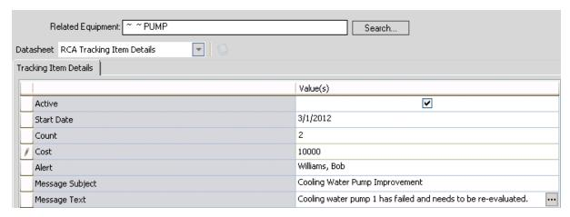
The value 2 in the Count field indicates that if the number of Failure records linked to the Equipment record *Pump* exceeds two, the alert email will be sent to Bob Williams. Note also that in the Cost field, the value 45 indicates that if the sum of the failure cost exceeds \$10,000, the alert email will be sent to Bob Williams.
