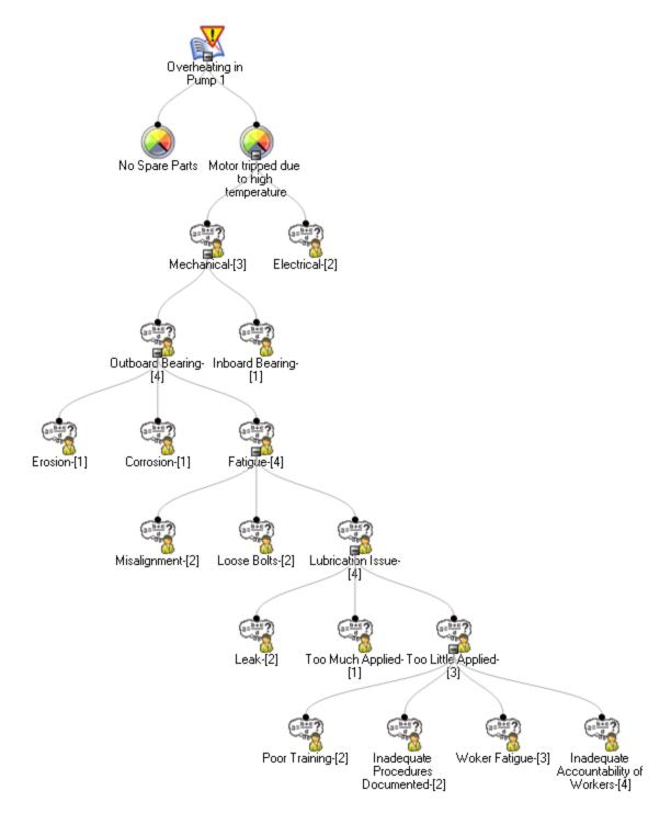
In the Logic Tree in this image, you can see that two Failure Mode nodes are linked to the Failure Event node, and multiple Hypothesis nodes are linked to the *Motor Tripped due to high temperature* Failure Mode node.
