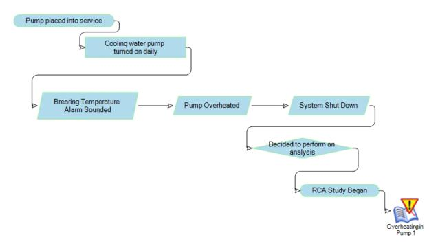
3. Diagram each failure mode in detail. For this example, you would create a Logic Tree like the one shown in the following image.
