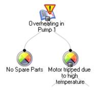
A given failure event can have multiple failure modes. For example, the image shows the failure modes from our Cooling Water Pump failure example. The Failure Event node (i.e., the overheated pump) is associated with the following Failure Mode nodes:
