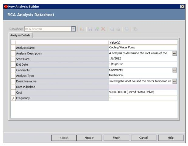
In the **Frequency of Failures** text box, the number 1 represents the number of failures that occurred for the cooling water pump.
