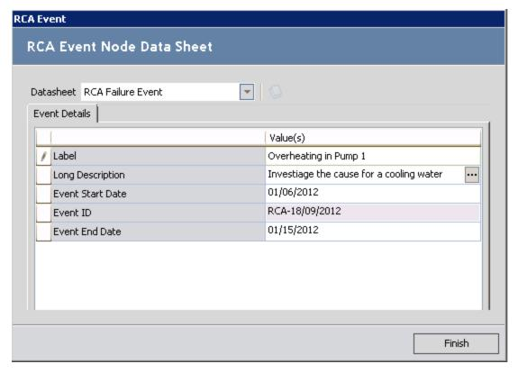
Each RCA Analysis will have one Failure Event node, which will always appear at the root level of the Logic Tree hierarchy and as the first node in the Event Diagram. For example, the following image shows the Failure Event node as it appears in the Logic Tree in our Cooling Water Pump example.
