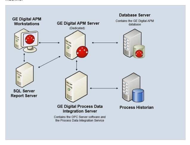
The following image shows the alternate configuration of these machines when the OPC Server software is installed on a *separate* machine from the Meridium APM Process Data Integration Service.
