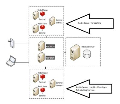
The following image illustrates how the Redis server setup used by GE Digital APM Scheduling Service communicates with instances of GE Digital APM over web socket protocol.
