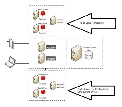
The following image illustrates how the Redis server setup used by Meridium Scheduling Service communicates with instances of Meridium Enterprise APM over web socket protocol.
