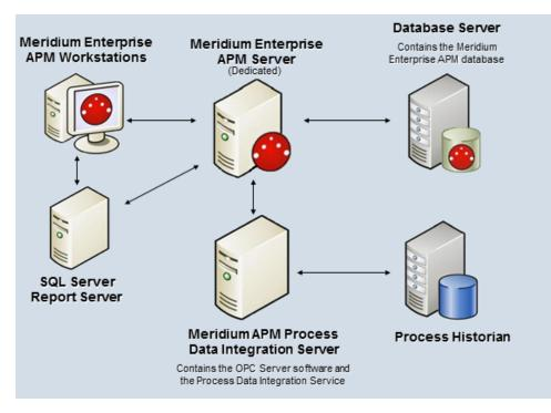
The following image shows the alternate configuration of these machines when the OPC Server software is installed on a *separate* machine from the Meridium APM Process Data Integration Service.
