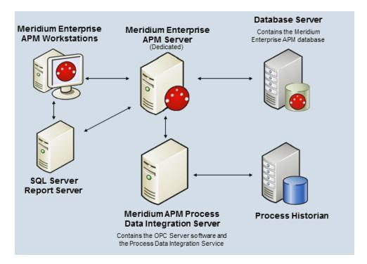
The following image shows the alternate configuration of these machines when the OPC Server software is installed on a *separate* machine from the Meridium APM Process Data Integration Service.
