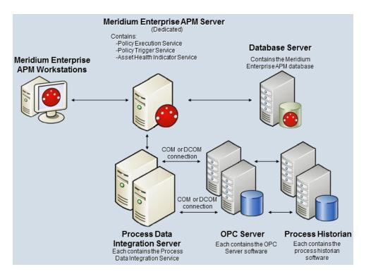
In either of these scenarios, when you complete the <u>first-time deployment steps for PDI</u>, you must install and configure the Process Data Integration Service on *each* Process Data Integration Server machine.
