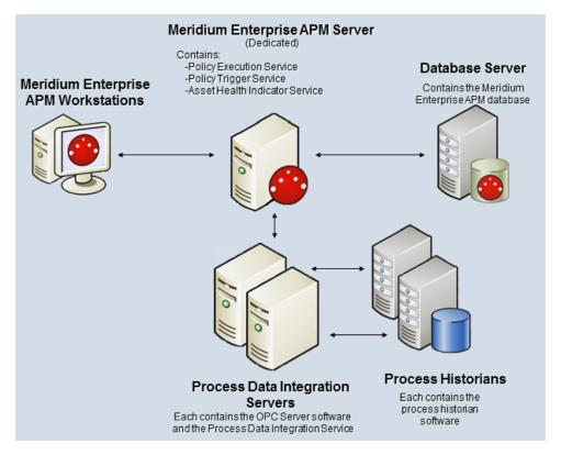
The following diagram illustrates multiple OPC Servers in an alternative configuration where the OPC Servers are separate machines from the PDI Servers.
