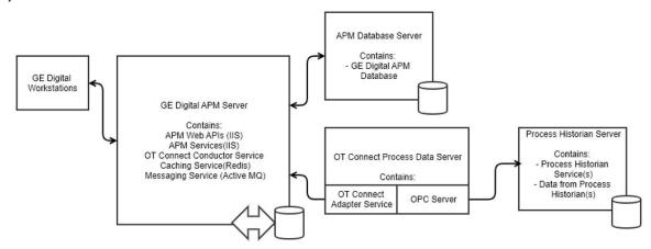
The Conductor requires access to the GE Digital APM Datasource(s), so it should be installed on the GE Digital APM Server with the other services.
