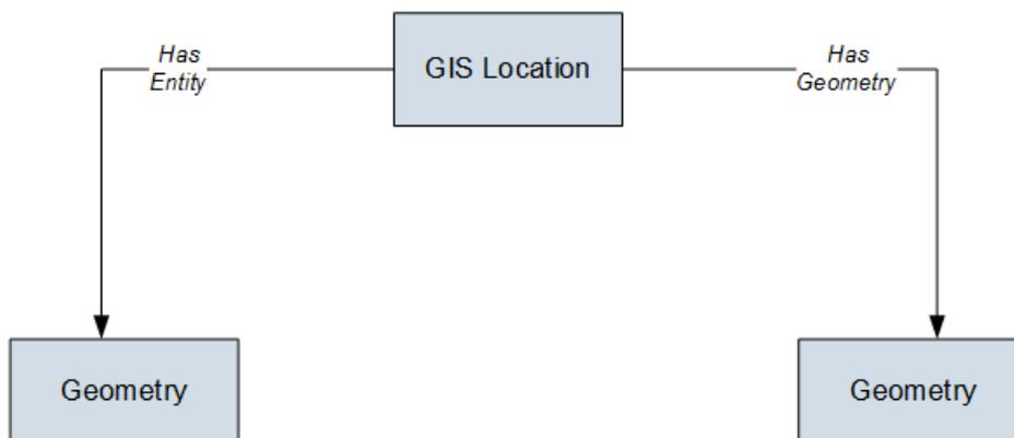
**Note:** In the diagram, GIS Location refers to the name of a database table. You can relate each GIS Location to an Entity of any family in GE Digital APM. Geometry represents the actual data for GIS Location. The Has Entity and Has Geometry are not relationship families defined in GE Digital APM.
