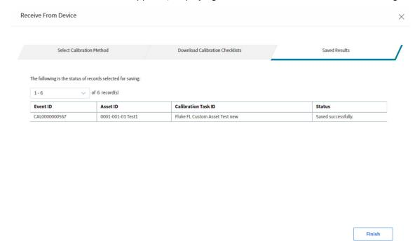
After receiving the calibration data, APM creates a Calibration record for each calibration that you have selected. If you have used a documenting process calibrator for calibration, then the fields in the **Test Equipment** section of each Calibration record created are populated with the details of the calibrator.
