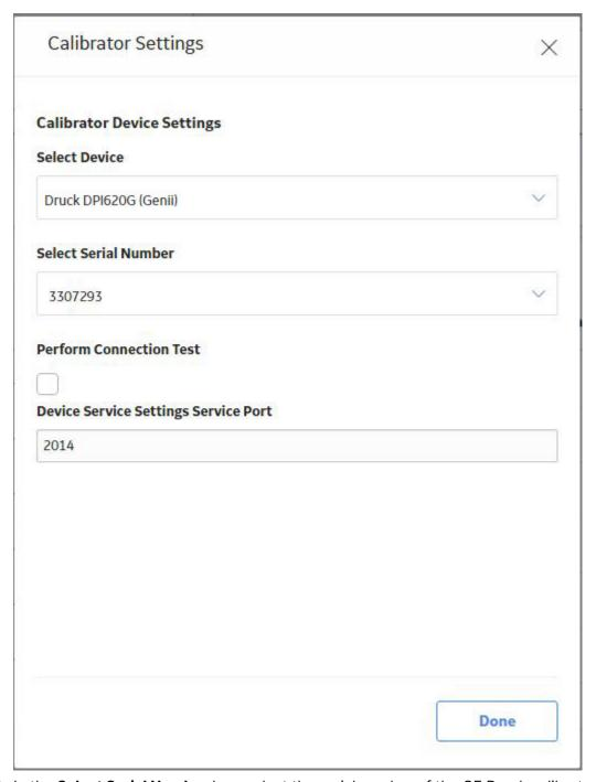
5. In the **Select Serial Number** box, select the serial number of the GE Druck calibrator.
