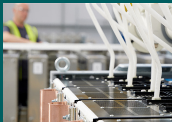
A technician working on Voltage-Sourced Converter valves in Stafford, United Kingdom
