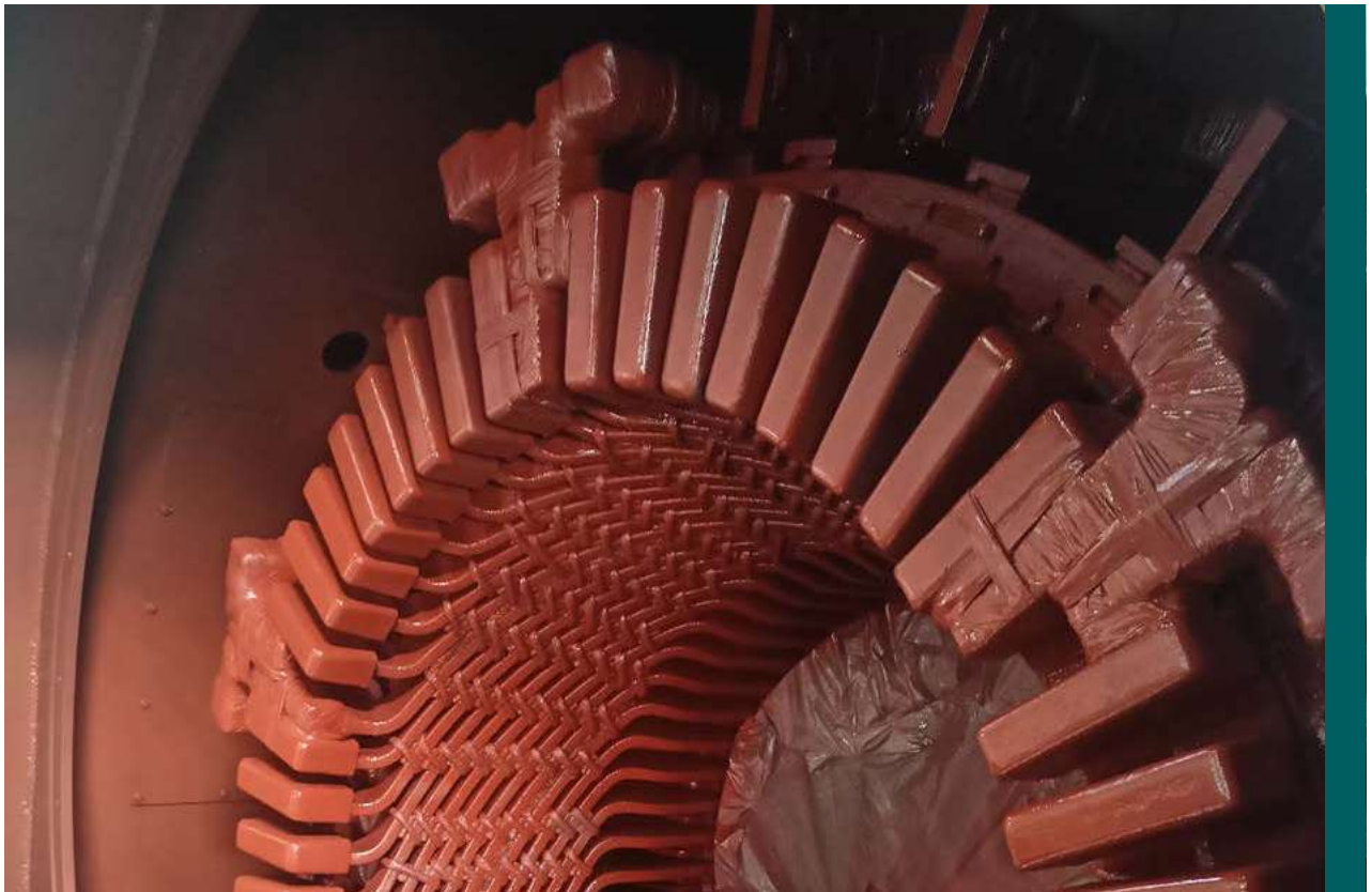
Full stator rewind of THRI- GVPI generator for Adhunik Power
