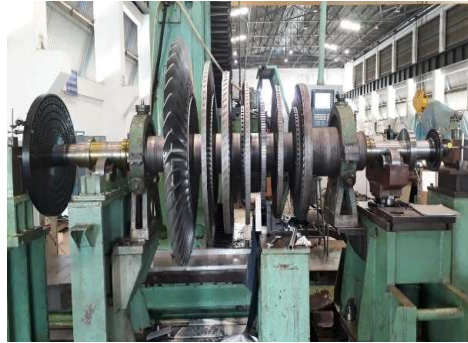
Rotor repair two 10.5 MW TDBFP rotors + 3 rd stage blade supply - Adani Power- Mundra plant
