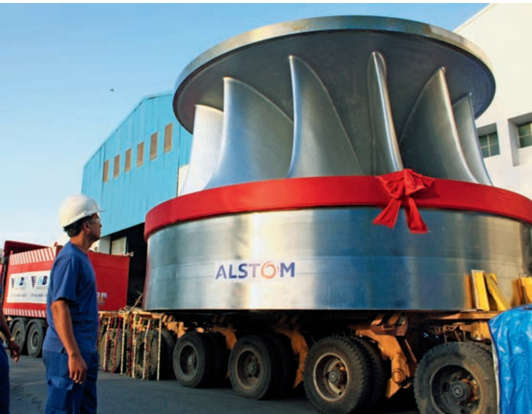
Biggest Francis Turbine Runner ever manufactured in India at Alstom Hydro Vadodara Workshop
