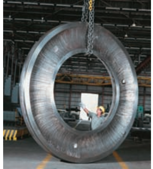
Grinding Ring of Coal Mill at Shahabad Workshop
