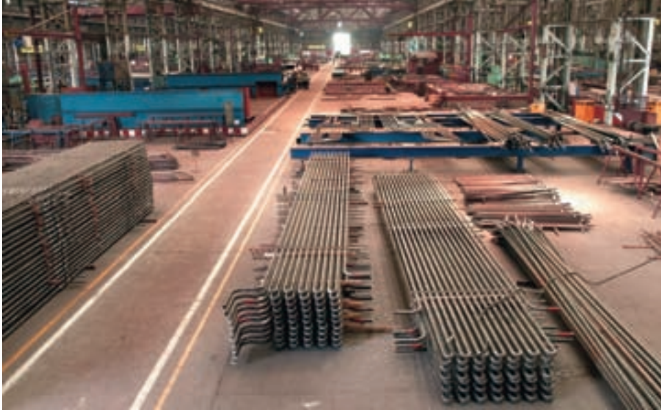
Panel under Fabrication at Durgapur Workshop
