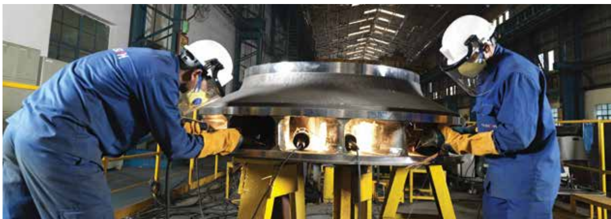
Francis Runner under work in progress at Hydro manufacturing site, Vadodara
