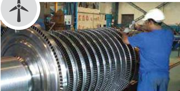
Blading activity for 210MW HP Rotor in progress at workshop in Vadodara
