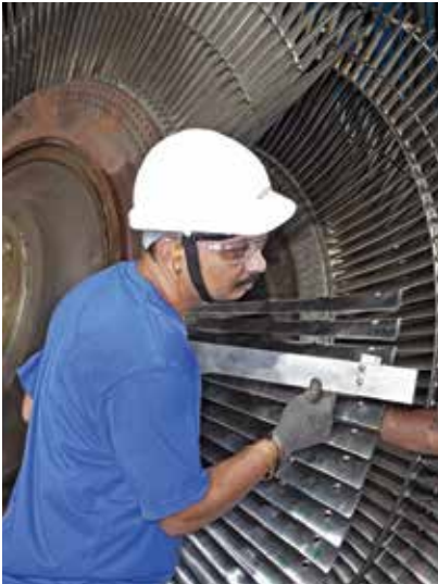
Thermal Services workshop at Vadodara LP, L-0 stage being bladed India, 2011
