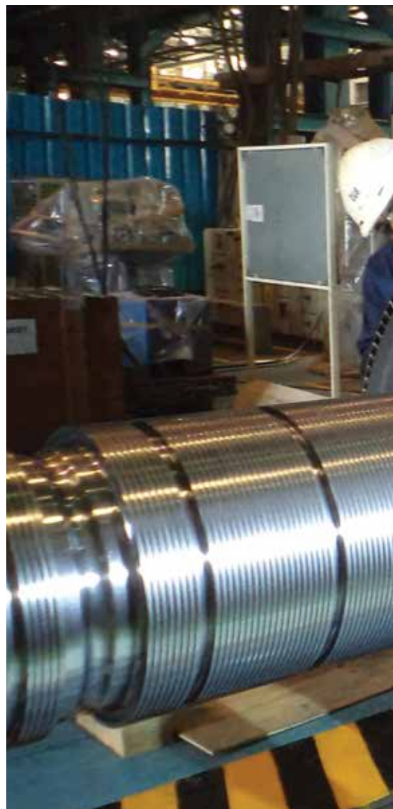
Blading activity for 210MW HP Rotor in progress at Thermal Serv
