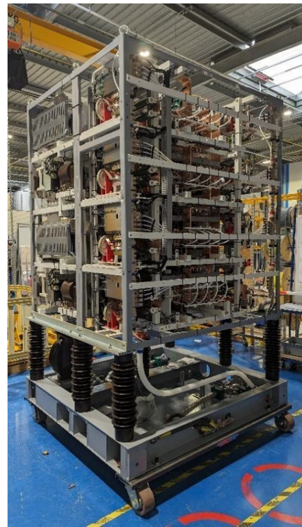
Fig. 7 MM7 HB Tower with 8 MMC cells
