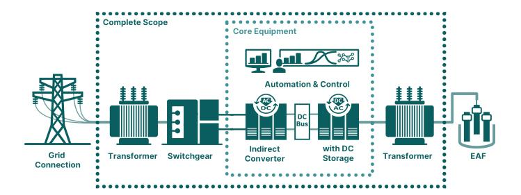
Compatible for both greenfield and brownfield as it can be located anywhere on site, usually close to the electrical substation,
