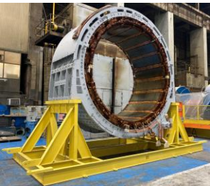
Complete Mag Frame for DC Motor GE 8000HP 850V 35/90RPM
