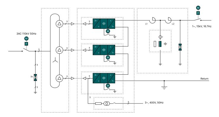
Circuit diagram of one converter block
