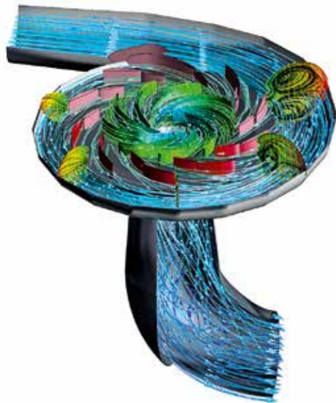
CFD calculation of pump-turbine runner CFD: computational fluid dynamics
