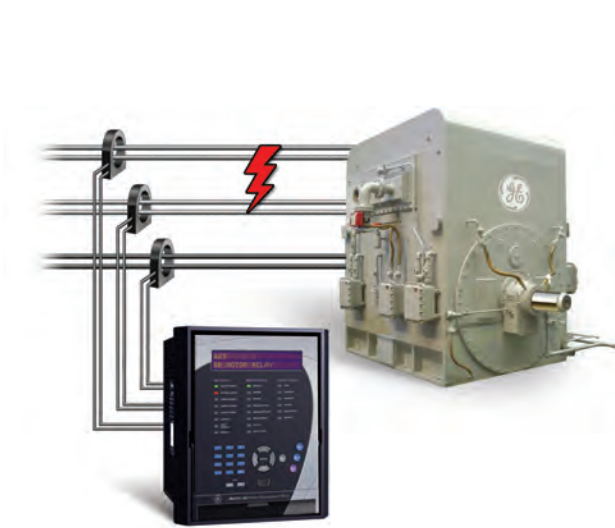
Figure 12. Differential protection of phase to phase faults
