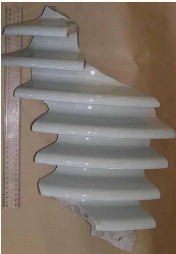
Fig. 3. Porcelain debris after rupture of a VT.
