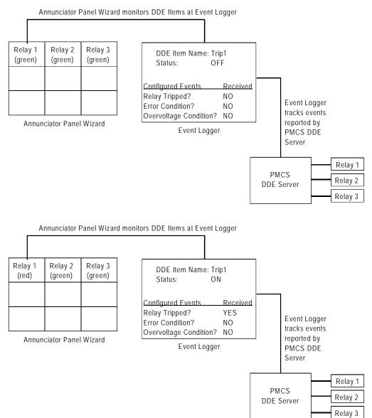
In the upper illustration, the Event Server watches for any of the three events configured to cause a change of state to the Trip 1 DDE Item. None of these three events has occurred, so the status of the Trip 1 DDE Item is at OFF. The Annunciator Panel wizard is monitoring the configured DDE Items at the Event Server, but all DDE Items are "OFF" so the Annunciator Panel displays green indicator tiles.
