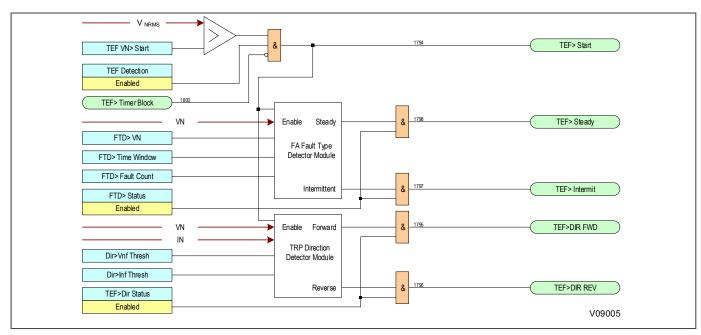
Figure 297: Transient Earth Fault Logic Overview
