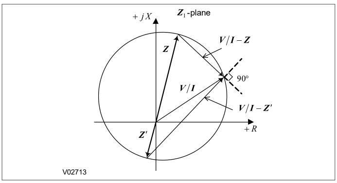
Figure 46: Offset Mho characteristics - impedance domain
