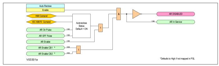
Figure 226: Autoreclose Enable logic diagram (Module 5)
