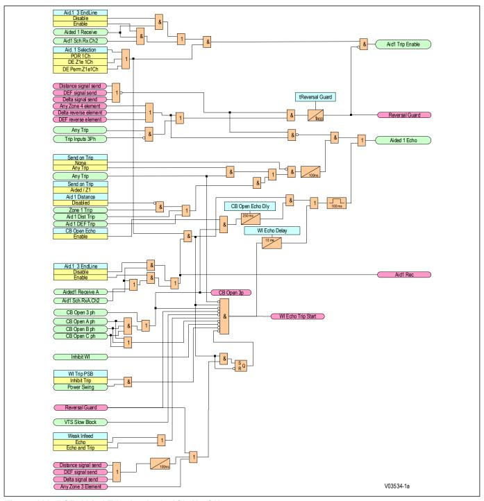
Figure 126: POR Aided Tripping logic 1Ch (1 of 2)
