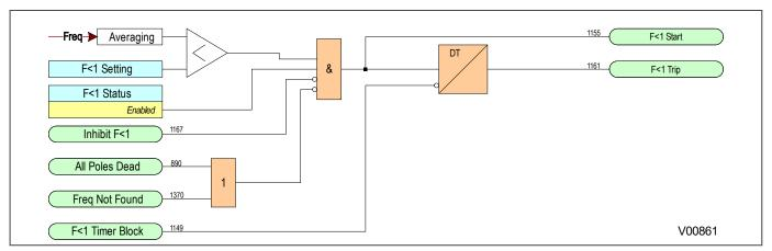
Figure 308: Underfrequency logic (single stage)
