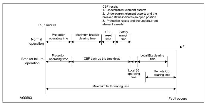
Figure 278: CB Fail timing
