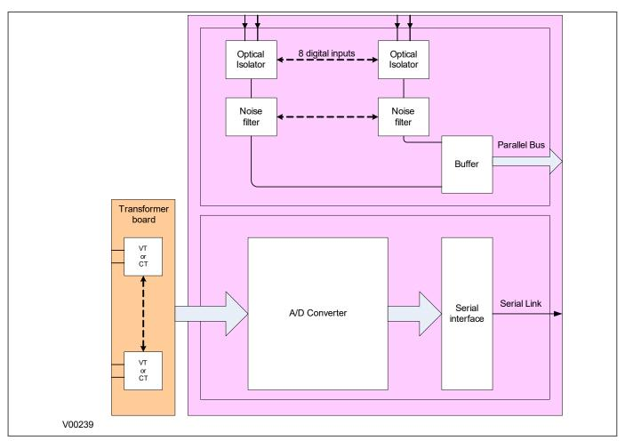
Figure 21: Input module schematic
