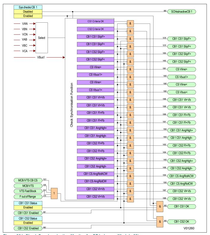
Figure 264: Check Synchronisation Monitor for CB1 closure (Module 60)
