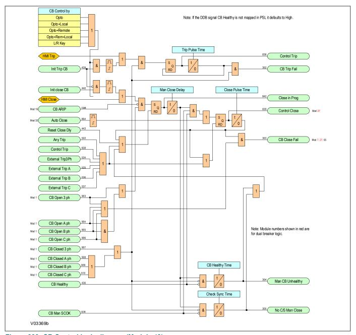
Figure 339: CB Control logic diagram (Module 43)
