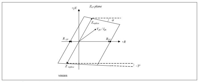
Figure 60: General characteristic in Z<sub>LP</sub> plane
