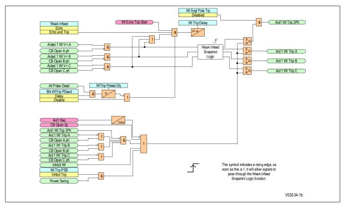
Figure 112: POR Aided Tripping logic 1Ch (2 of 2) – Weak Infeed Trip
