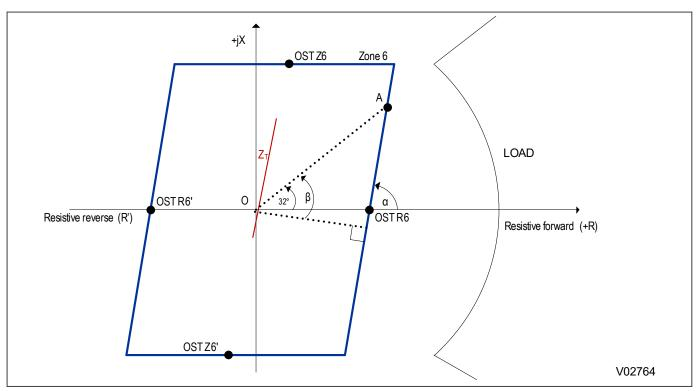
Figure 178: R6<sub>MAX</sub> determination
