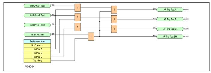
Figure 194: Autoreclose Trip Test logic diagram (Module 12)
