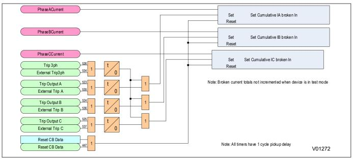
Figure 319: Broken Current Accumulator logic diagram
