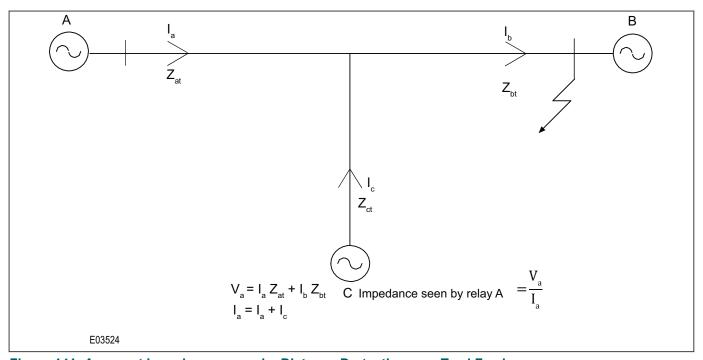
Figure 141: Apparent Impedances seen by Distance Protection on a Teed Feeder
