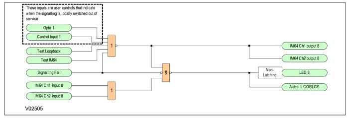
Figure 372: IM64 two-terminal scheme extended supervision
