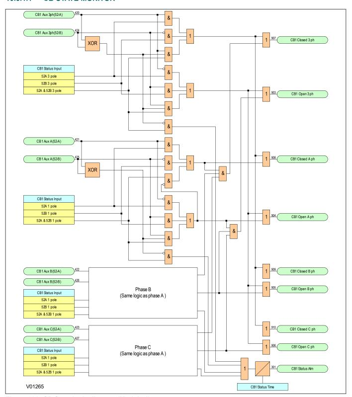
Figure 222: CB State logic diagram (Module 1)
