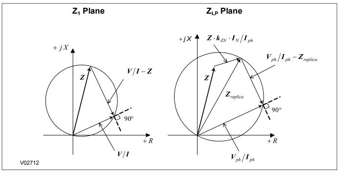
Figure 45: Directional Mho element construction - impedance domain
