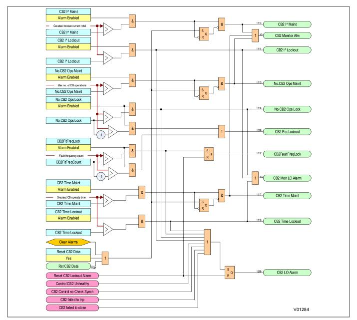
Figure 331: CB2 Condition Monitoring logic diagram
