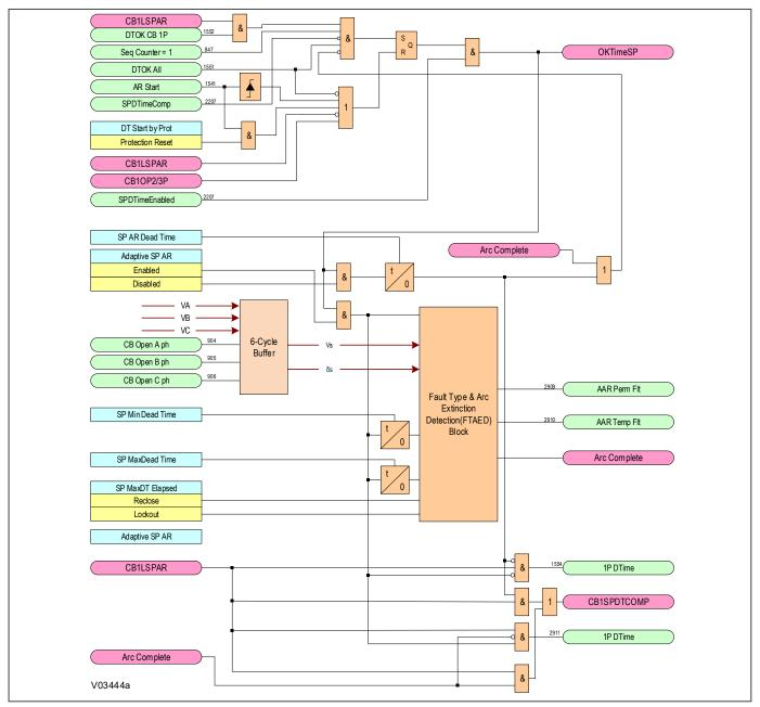
Figure 203: Single-phase Dead Time logic diagram (Module 24)
