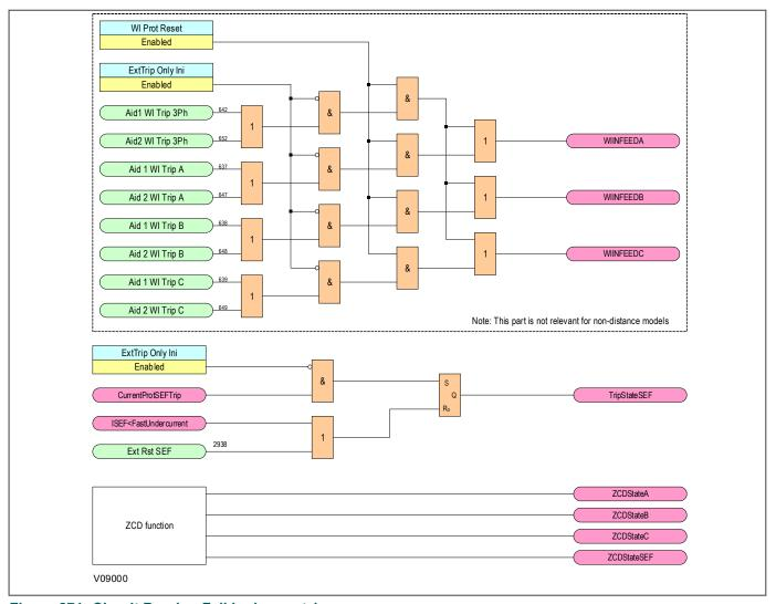
Figure 271: Circuit Breaker Fail logic - part 1
