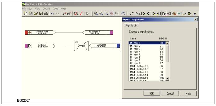
Figure 374: Example assignment of InterMiCOM signals within the PSL
