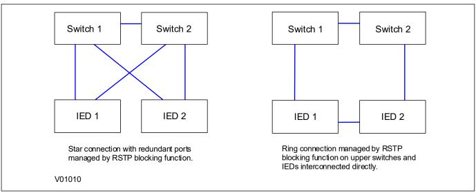
Figure 384: IED attached to redundant Ethernet star or ring circuit
