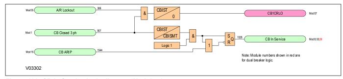
Figure 188: CB In Service logic diagram (Module 4)
