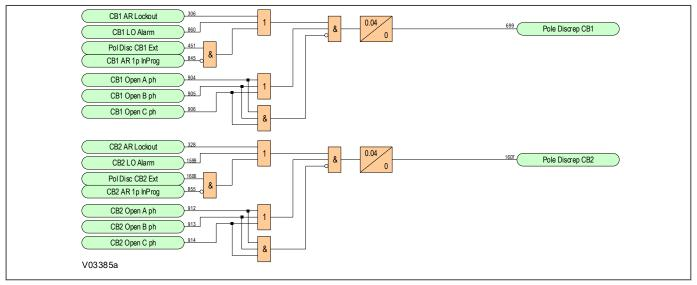
Figure 261: Pole Discrepancy Logic Diagram (Module 62)
