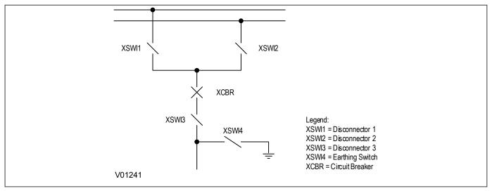
Figure 352: Representation of typical feeder bay
