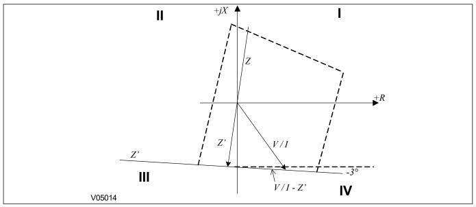
Figure 65: Reverse impedance reach line construction
