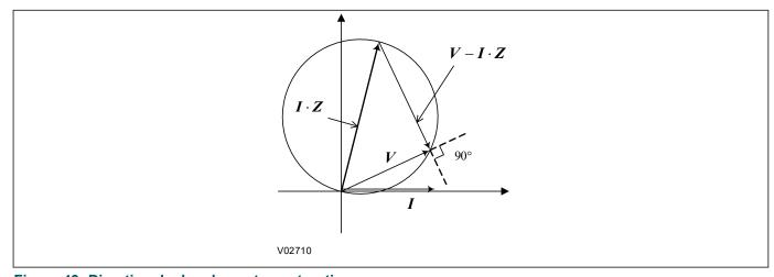
Figure 43: Directional mho element construction
