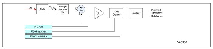
Figure 298: Fault Type Detector Logic
