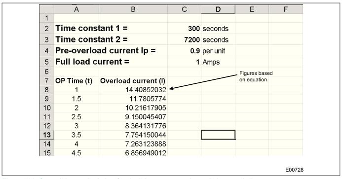
Figure 292: Spreadsheet calculation for dual time constant thermal characteristic
