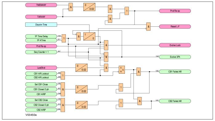
Figure 235: Protection Reoperation and Evolving Fault logic diagram (Module 20)
