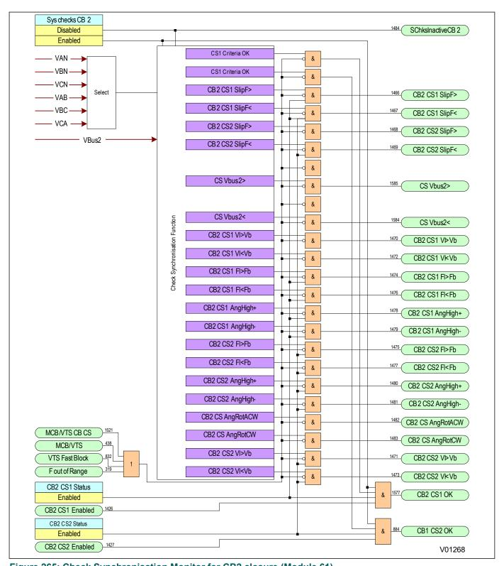
Figure 265: Check Synchronisation Monitor for CB2 closure (Module 61)
