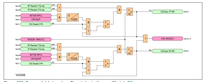
Figure 208: Successful Autoreclose Signals logic diagram (Module 36)
