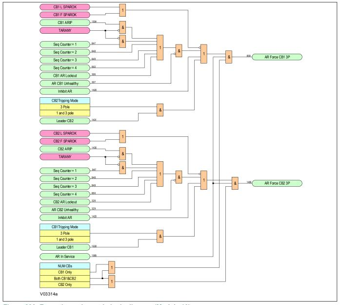
Figure 230: Force three-phase trip logic diagram (Module 10)
