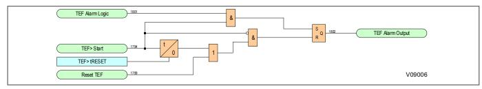
Figure 300: TEFD output alarm logic
