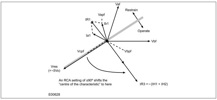
Figure 287: Phasor diagrams for insulated system with C phase fault
