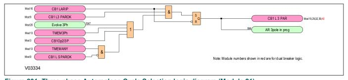
Figure 201: Three-phase Autoreclose Cycle Selection logic diagram (Module 21)
