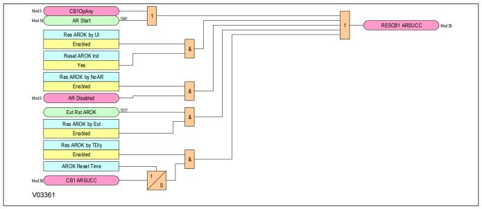
Figure 209: Autoreclose Reset Successful Indication logic diagram (Module 37)
