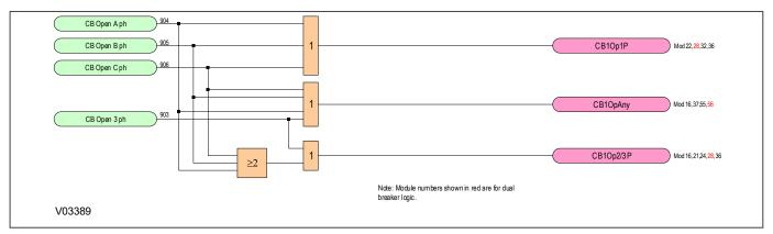
Figure 187: Circuit Breaker Open logic diagram (Module 3)
