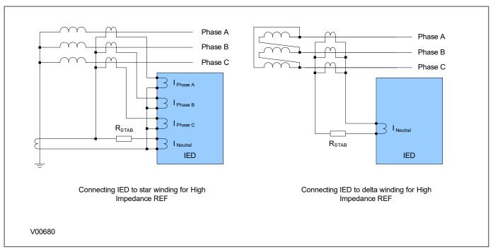
Figure 290: High impedance REF connection
