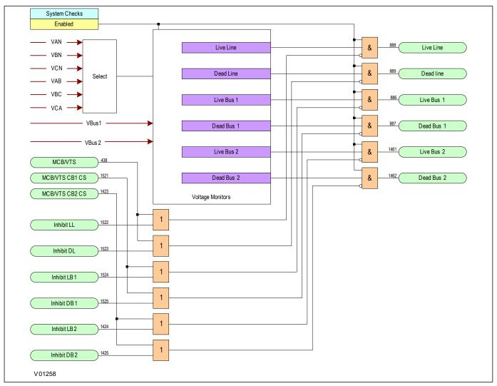
Figure 263: Voltage Monitor for CB Closure (Module 59)
