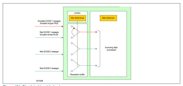
Figure 401: Simulated input behaviour
