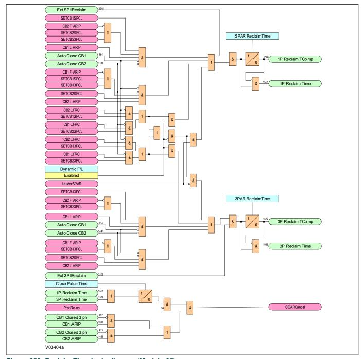
Figure 250: Reclaim Time logic diagram (Module 35)
