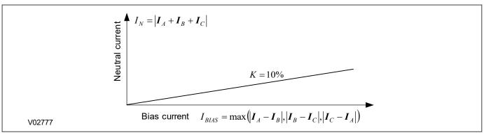
Figure 74: Biased Neutral Current Detector Characteristic
