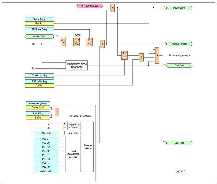
Figure 167: Power swing blocking logic
