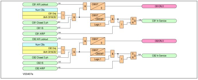
Figure 225: CB In Service logic diagram (Module 4)
