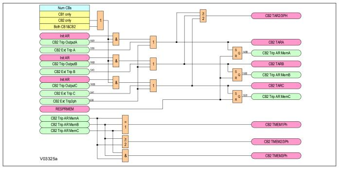
Figure 234: Autoreclose initiation by internal single and three phase trip or external trip for CB2 (Module 14)
