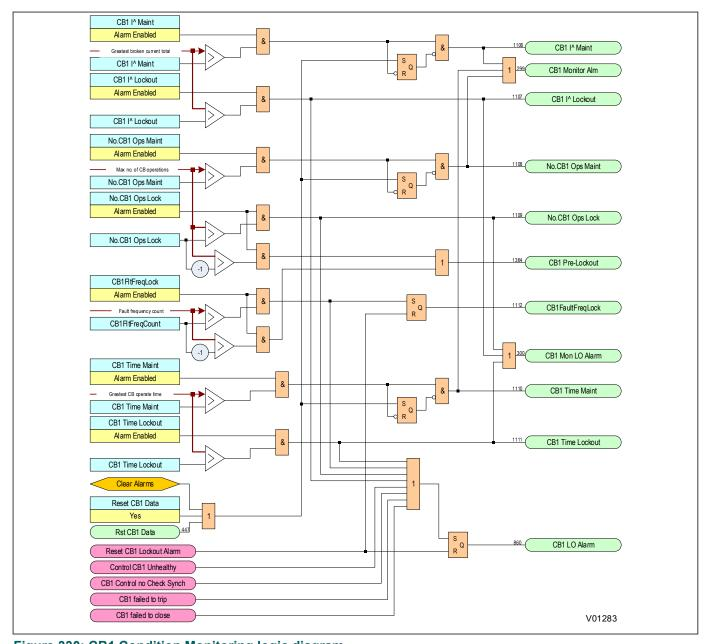
Figure 330: CB1 Condition Monitoring logic diagram
