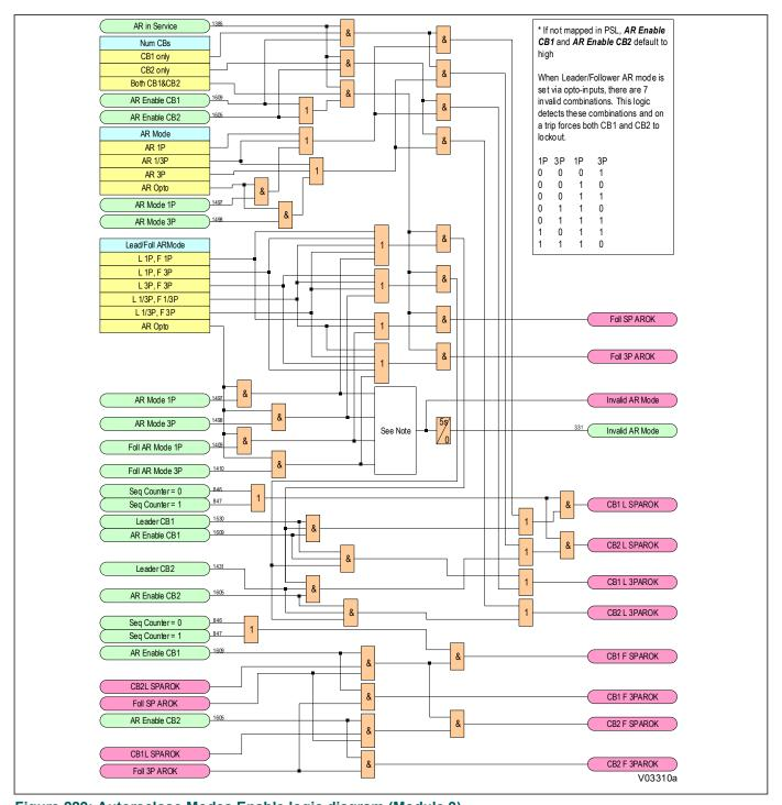
Figure 229: Autoreclose Modes Enable logic diagram (Module 9)
