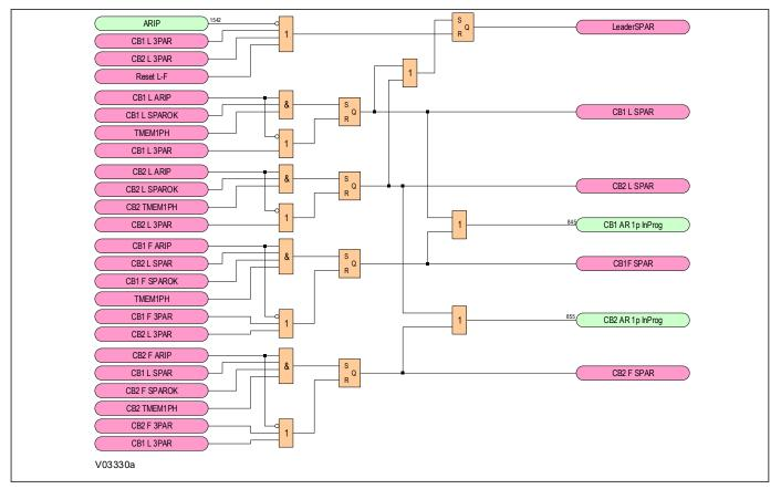
Figure 240: Single-phase Autoreclose Cycle Selection logic diagram (Module 19)
