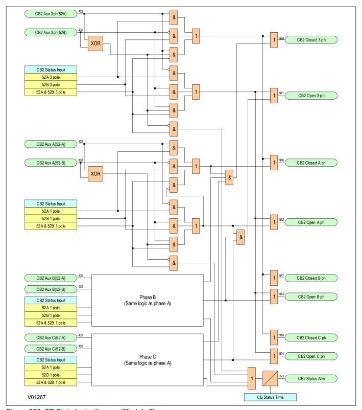
Figure 336: CB State logic diagram (Module 2)
