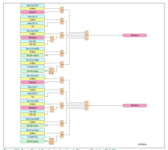
Figure 333: Reset Circuit Breaker Lockout Logic Diagram (Modules 57 & 58)
