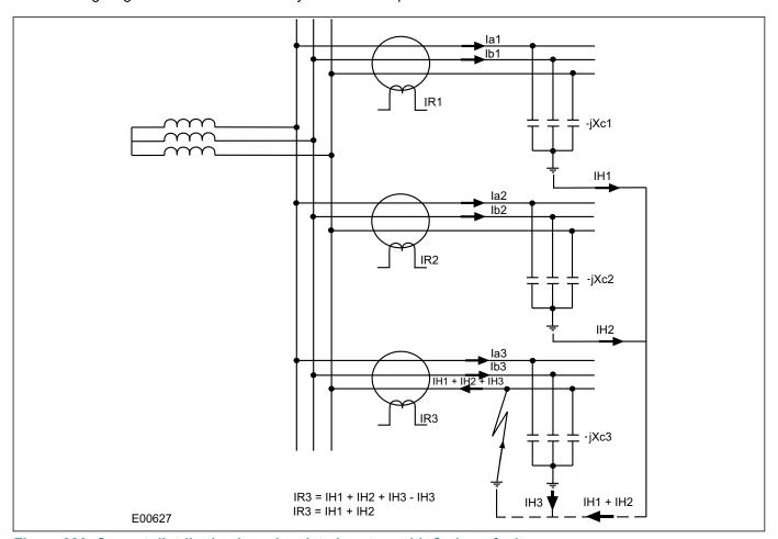
Figure 286: Current distribution in an insulated system with C phase fault
