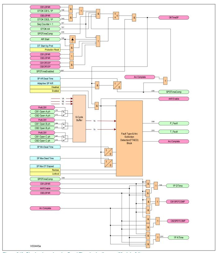
Figure 243: Single-phase Leader Dead Time logic diagram (Module 24)
