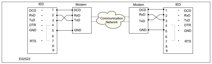
Figure 376: Indirect connection using modems
