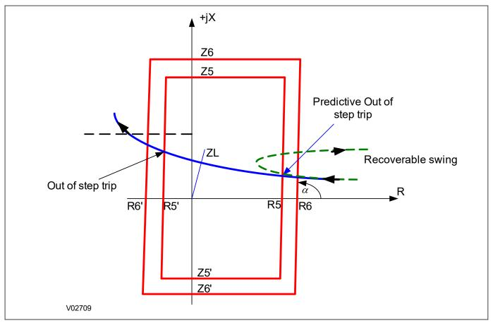
Figure 164: Out of step detection characteristic
