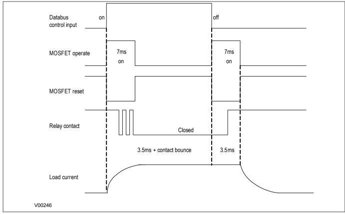
Figure 26: High Break contact operation
