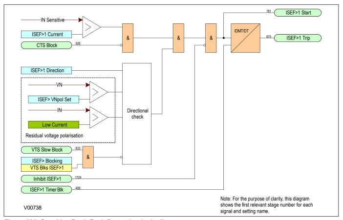
Figure 285: Sensitive Earth Fault Protection logic diagram
