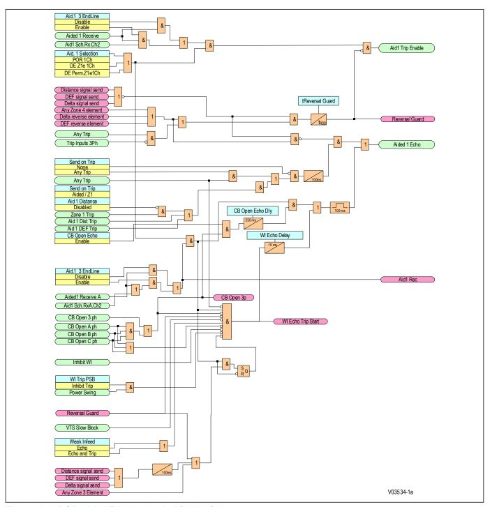
Figure 136: POR Aided Tripping logic 1Ch (1 of 2)
