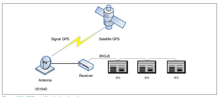
Figure 390: GPS satellite timing signal
