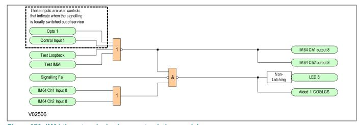
Figure 373: IM64 three-terminal scheme extended supervision
