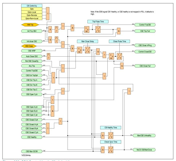
Figure 256: CB2 Control Logic (Module 44)
