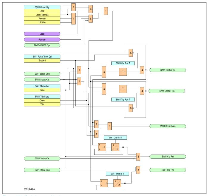
Figure 355: Switch control logic
