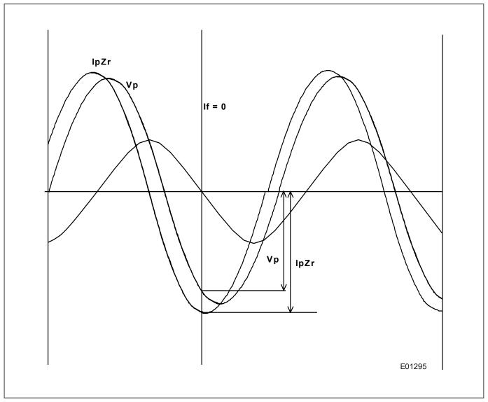
Figure 318: Fault locator selection of fault current zero
