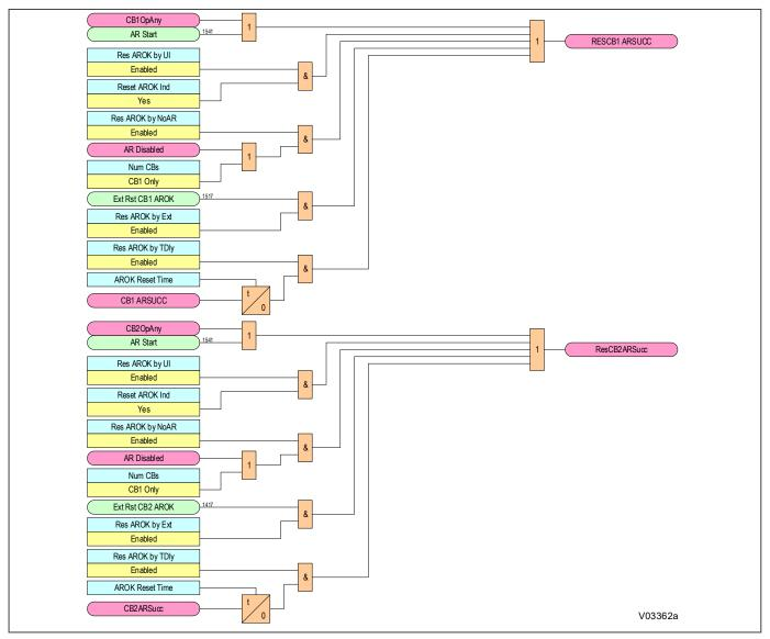
Figure 252: Autoreclose Reset Successful Indication logic diagram (Modules 37 & 38)
