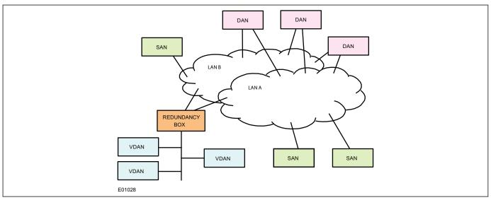
Figure 380: Example PRP redundant network
