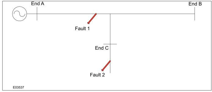
Figure 142: POR tee feeder fault example
