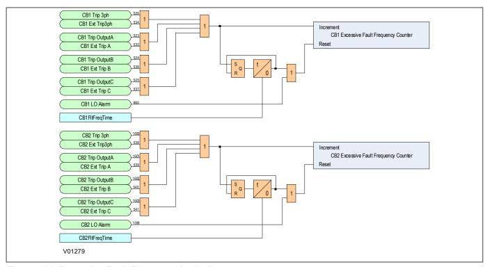
Figure 326: Excessive Fault Frequency logic diagram
