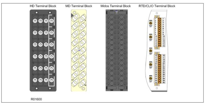
Figure 406: Possible terminal block types
