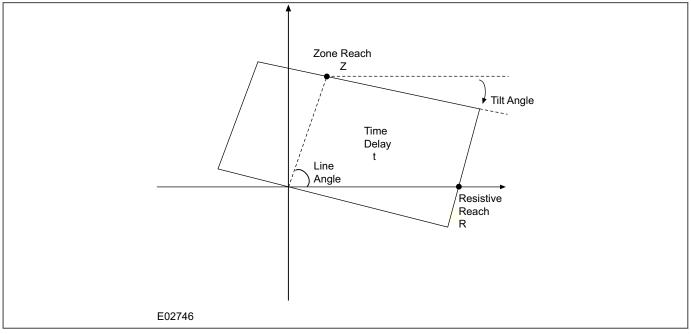
Figure 92: Settings required to apply a quadrilateral zone
