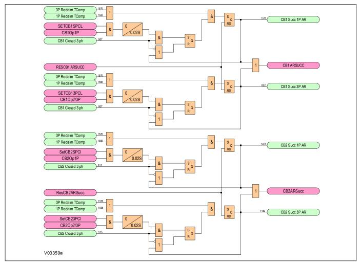
Figure 251: Successful Autoreclose Signals logic diagram (Module 36)
