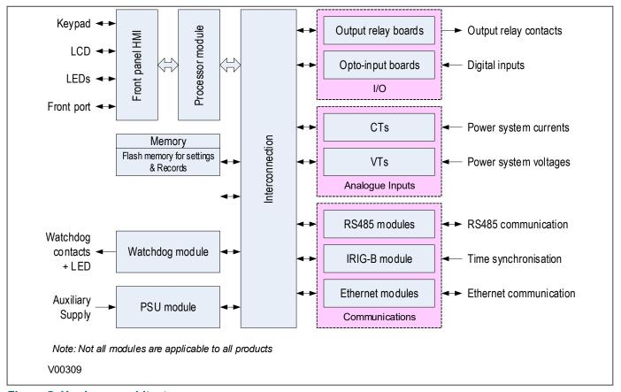
Figure 5: Hardware architecture
