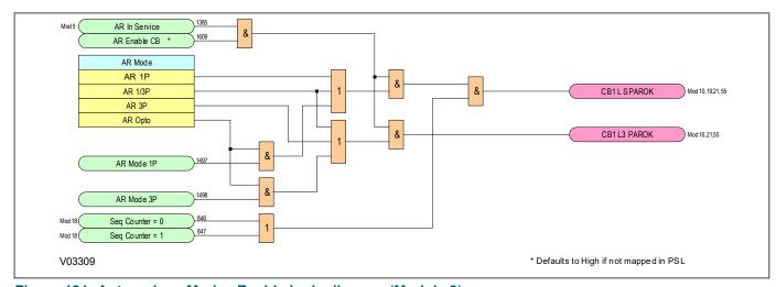
Figure 191: Autoreclose Modes Enable logic diagram (Module 9)
