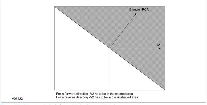
Figure 119: Directional criteria for residual voltage polarization
