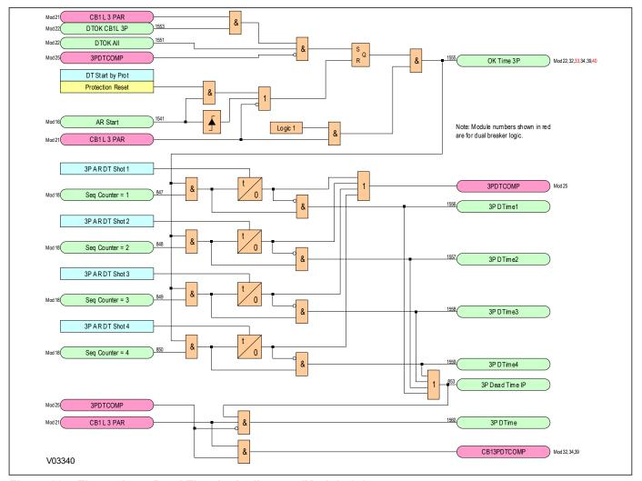
Figure 204: Three-phase Dead Time logic diagram (Module 25)
