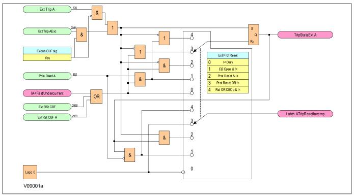
Figure 272: Circuit Breaker Fail logic - part 2
