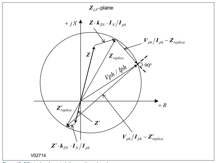
Figure 47: Offset mho characteristics – voltage domain
