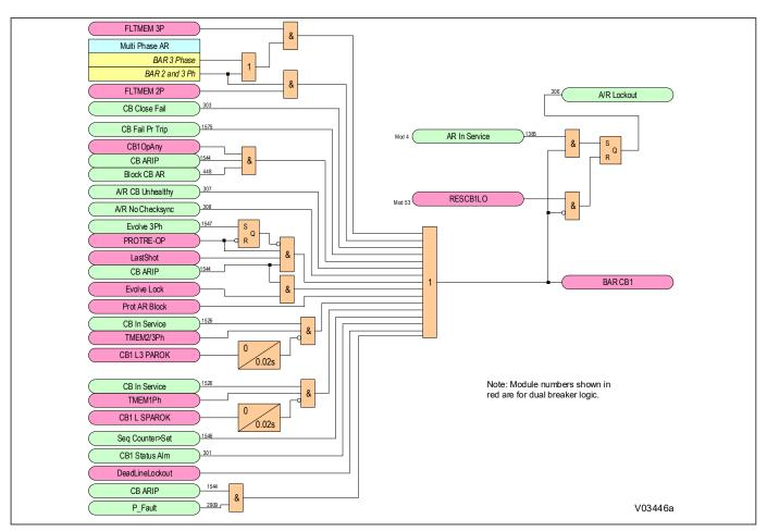
Figure 214: AR Lockout Logic Diagram (Module 55)
