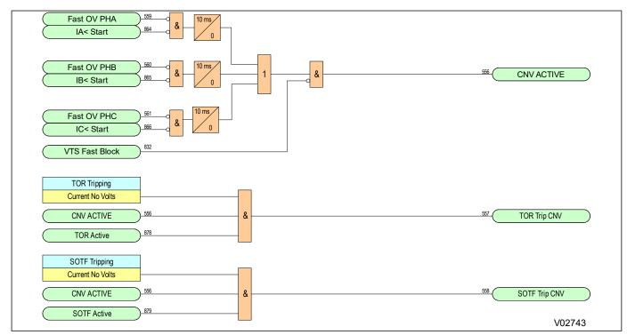
Figure 149: Trip On Close based on CNV level detectors
