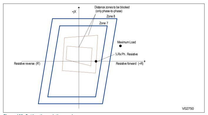
Figure 168: Setting the resistive reaches
