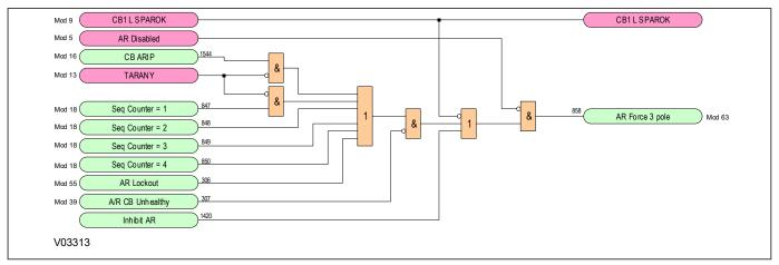
Figure 192: Force Three-phase Trip logic diagram (Module 10)
