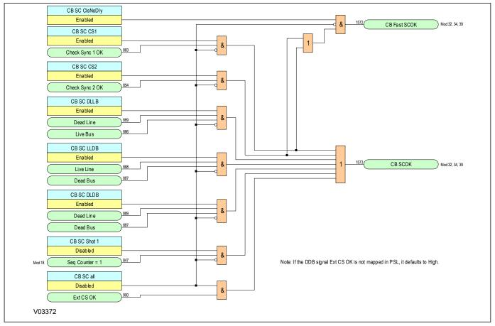
Figure 220: Three-phase Autoreclose System Check Logic Diagram (Module 45)
