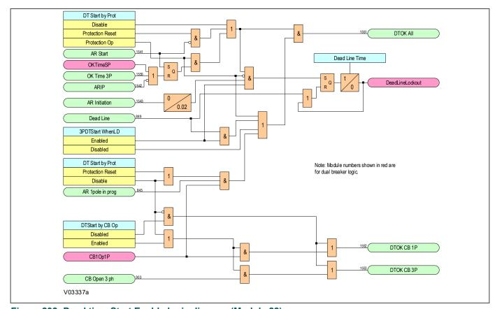
Figure 202: Dead time Start Enable logic diagram (Module 22)
