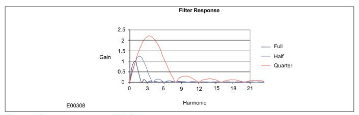
Figure 34: Frequency response of FIR filters
