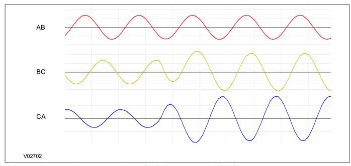
Figure 73: Phase to phase current changes for C phase-to-ground (CN) fault
