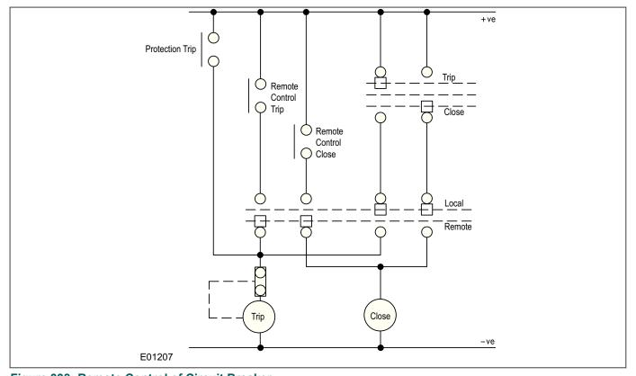
Figure 338: Remote Control of Circuit Breaker
