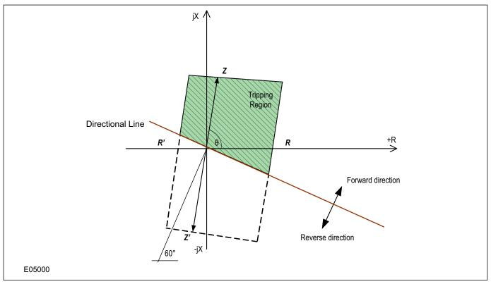
Figure 55: Directional Quadrilateral Characteristic
