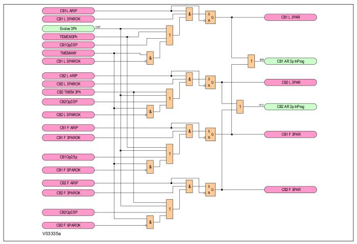
Figure 241: Three-phase Autoreclose Cycle Selection logic diagram (Module 21)
