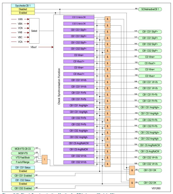
Figure 348: Check Synchronisation Monitor for CB1 closure (Module 60)
