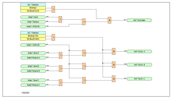
Figure 129: Aided Scheme Blocking 1 Tripping logic
