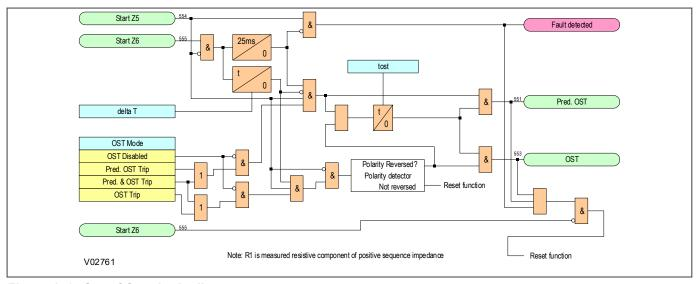
Figure 172: Out of Step logic diagram
