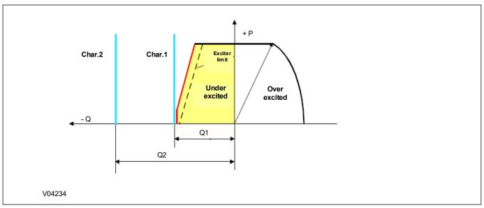
Figure 313: Reactive power protection for underexcitation protection
