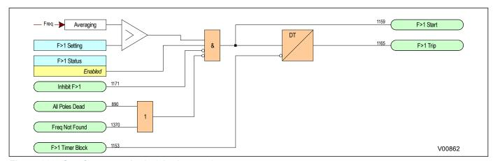
Figure 309: Overfrequency logic (single stage)
