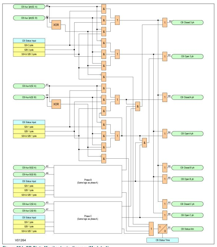
Figure 334: CB State Monitor logic diagram (Module 1)
