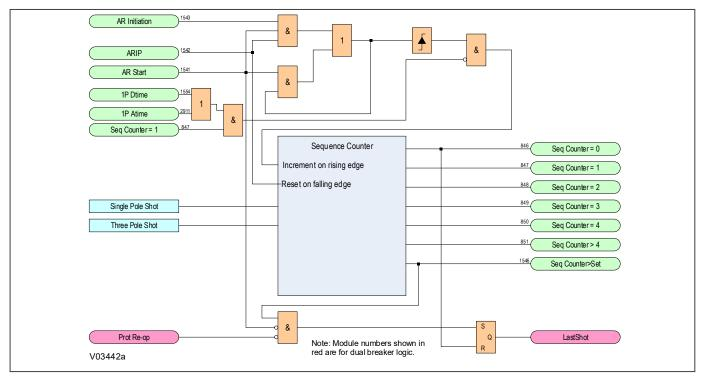
Figure 199: Autoreclose Sequence Counter logic diagram (Module 18)
