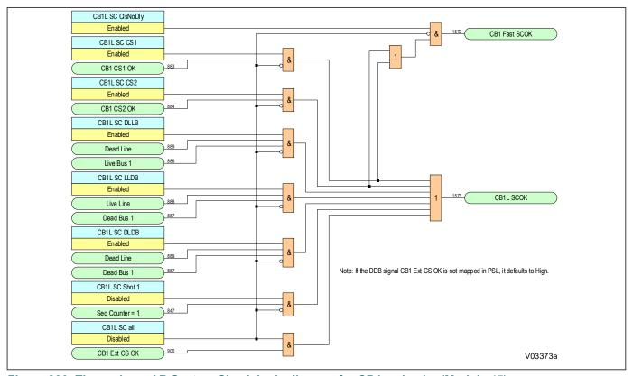
Figure 266: Three-phase AR System Check logic diagram for CB1 as leader (Module 45)
