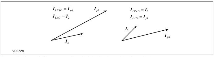
Figure 61: Phase relations between I2 and Iph for leading and lagging polarizing currents
