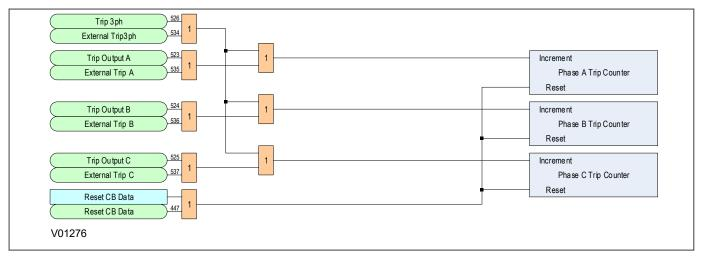
Figure 321: CB Trip Counter logic diagram
