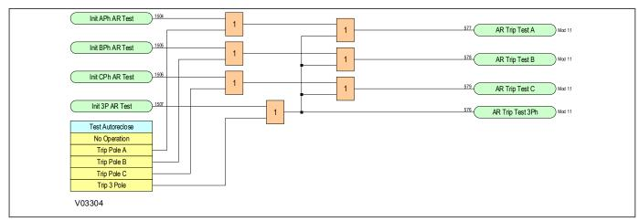
Figure 232: Autoreclose Trip Test logic diagram (Module 12)
