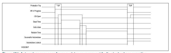
Figure 184: Autoreclose sequence for an evolving or permanent fault - single-phase operation
