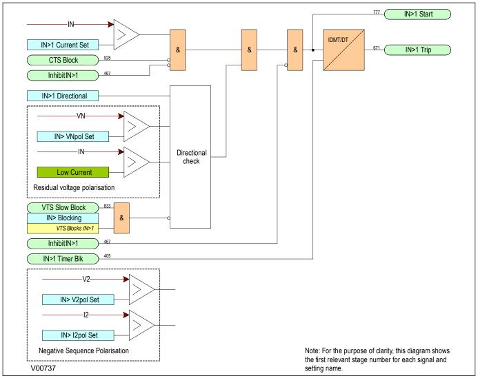
Figure 283: Earth Fault Protection logic diagram
