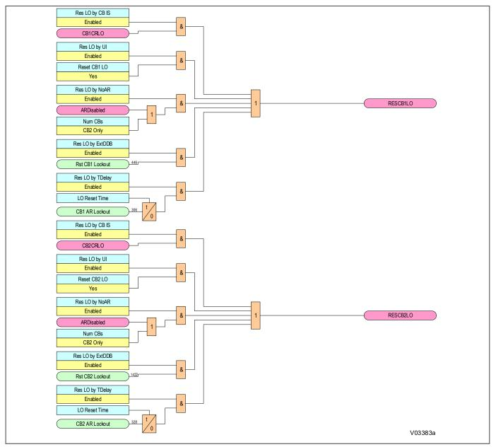
Figure 260: Reset Circuit Breaker Lockout Logic Diagram (Modules 57 & 58)
