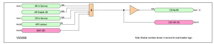
Figure 189: Autoreclose OK logic diagram (Module 8)
