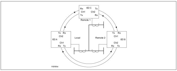
Figure 367: Fibre Teleprotection connections for a three-terminal Scheme
