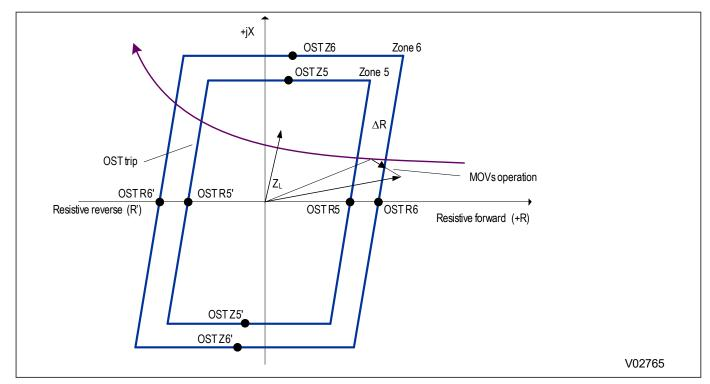
Figure 179: Example of timer reset due to MOV's operation
