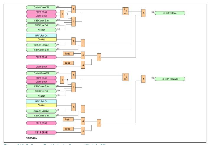
Figure 245: Follower Enable logic diagram (Module 27)
