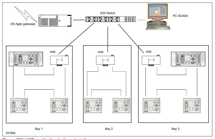
Figure 383: HSR application in the substation
