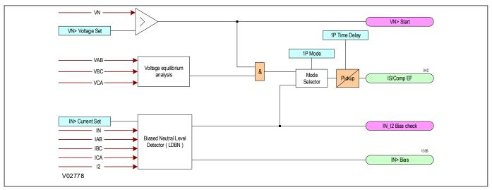
Figure 86: First earth fault detection
