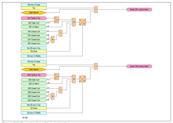
Figure 328: Reset Lockout Alarm logic diagram
