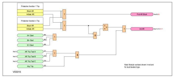
Figure 231: Autoreclose Initiation logic diagram (Module 11)
