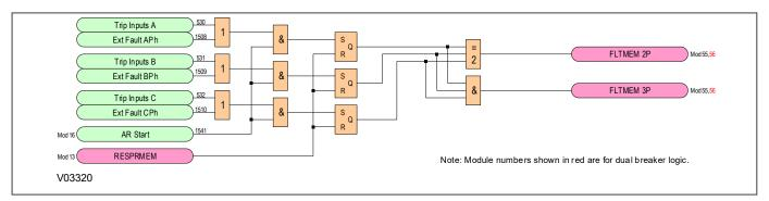
Figure 236: Fault Memory logic diagram (Module 15)
