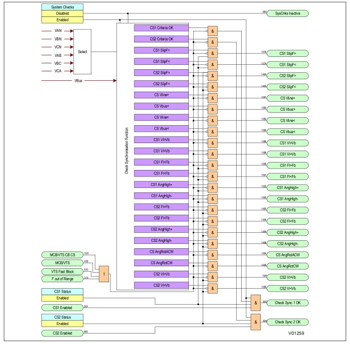
Figure 347: Check Synchronisation Monitor for CB closure (Module 60)
