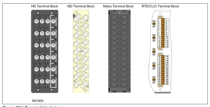
Figure 394: Terminal block types
