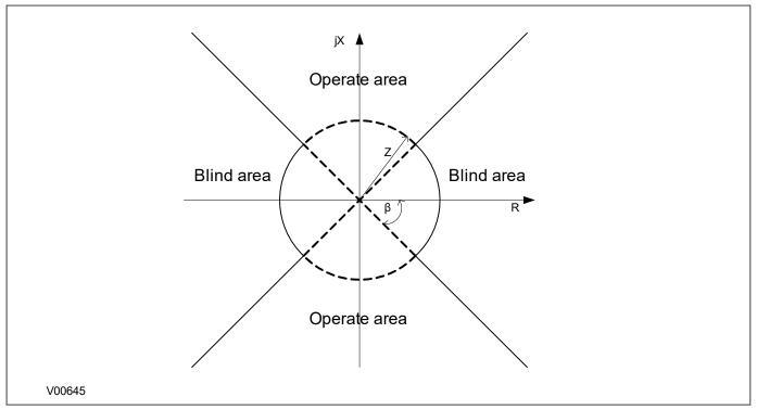
Figure 77: Load Blinder Characteristics
