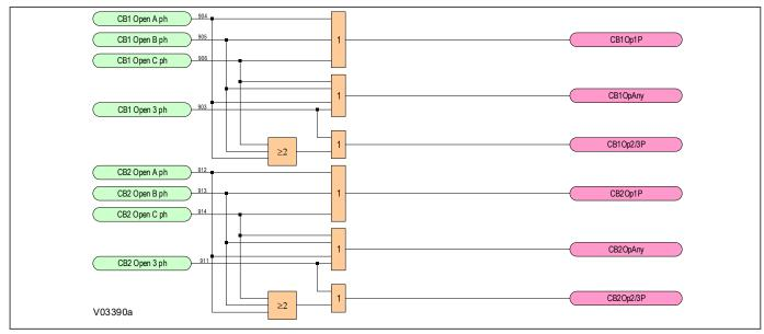
Figure 224: Circuit Breaker Open logic diagram (Module 3)
