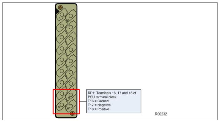
Figure 19: Rear serial port terminals
