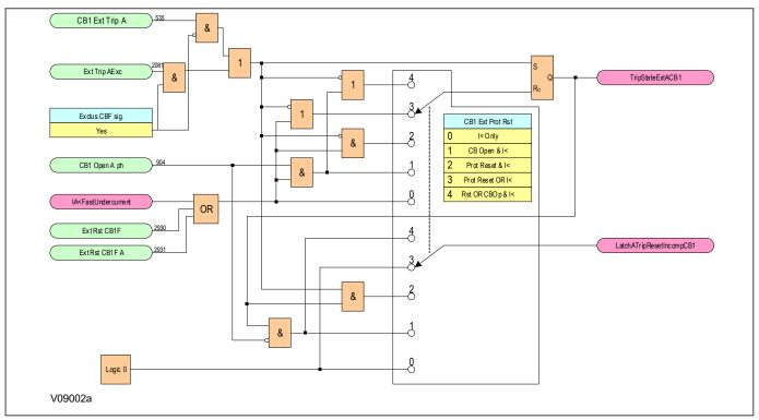
Figure 273: Circuit Breaker Fail logic - part 2
