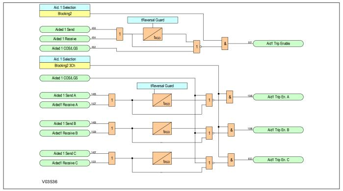
Figure 140: Aided Scheme Blocking 2 Tripping logic
