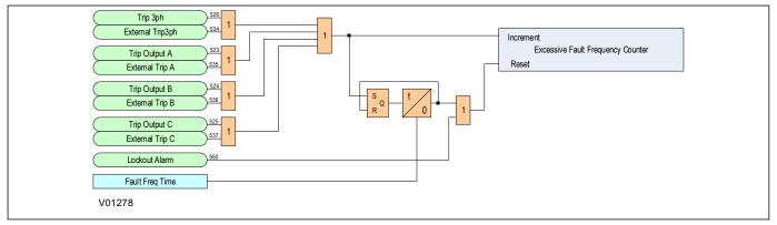
Figure 325: Excessive Fault Frequency logic diagram
