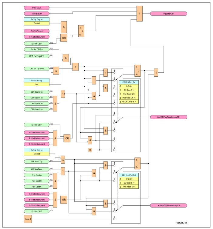
Figure 275: Circuit Breaker Fail logic - part 3
