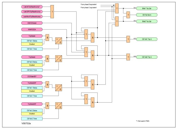
Figure 276: Circuit Breaker Fail logic - part 4
