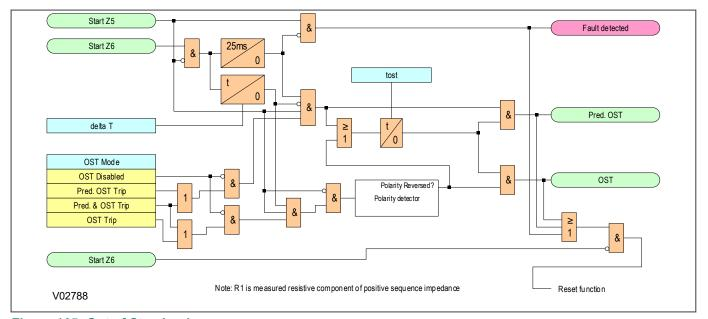
Figure 165: Out of Step Logic
