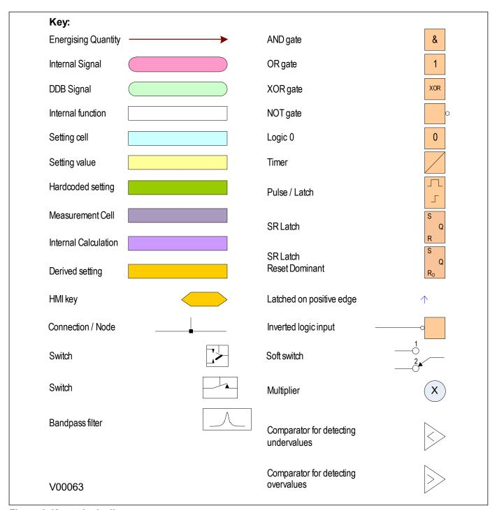
Figure 1: Key to logic diagrams
