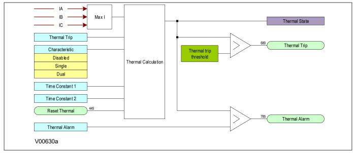
Figure 291: Thermal overload protection logic diagram
