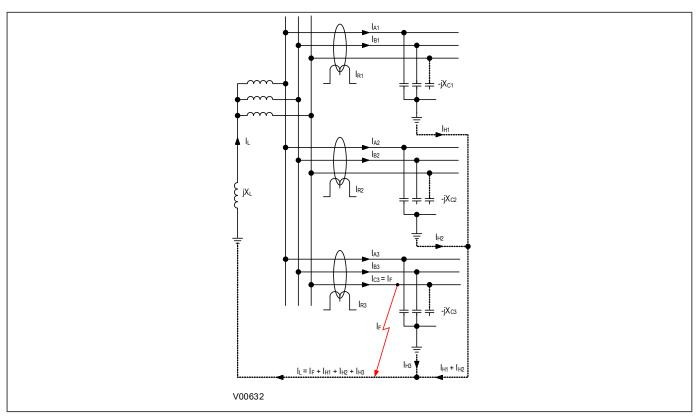
Figure 80: Distribution of currents during a Phase C fault
