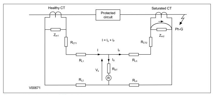
Figure 289: High impedance REF principle
