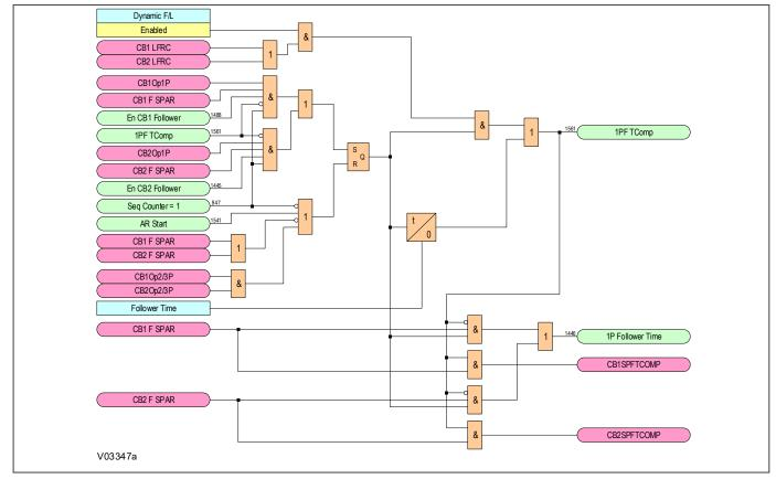
Figure 246: Single-phase Follower CB timing logic diagram (Module 28)
