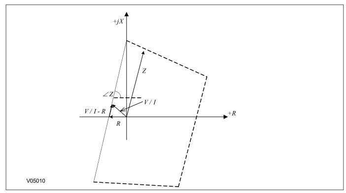
Figure 71: Reverse resistive reach line construction
