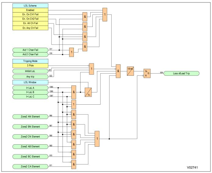
Figure 157: Loss of Load Logic
