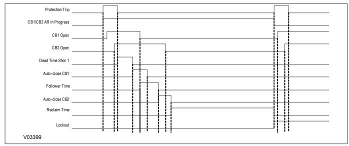
Figure 183: Autoreclose Sequence for an evolving/permanent fault on a dual CB application
