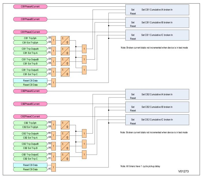
Figure 320: Broken Current Accumulator logic diagram
