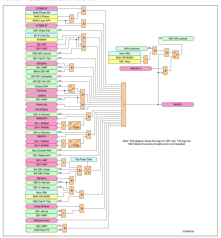
Figure 258: CB1 Lockout Logic Diagram (Module 55)
