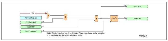
Figure 305: Residual Overvoltage logic
