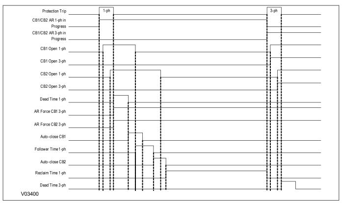
Figure 185: Autoreclose Sequence for a persistent fault on a multishot dual CB application set for single-phase operation
