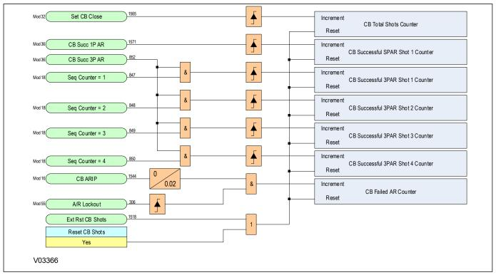
Figure 211: Autoreclose Shot Counters logic diagram (Module 41)
