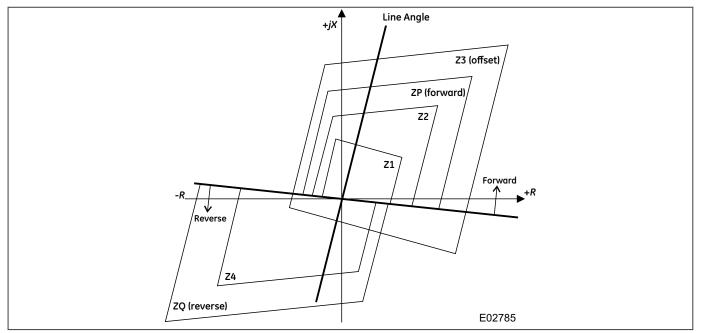
Figure 53: Simplified quadrilateral characteristics
