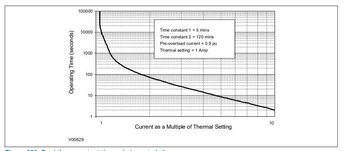
Figure 293: Dual time constant thermal characteristic
