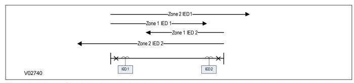
Figure 156: Loss of load accelerated trip scheme
