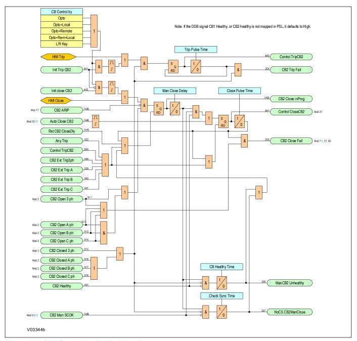
Figure 341: CB2 Control Logic (Module 44)
