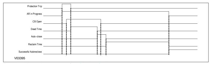
Figure 180: Autoreclose sequence for a Transient Fault
