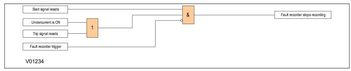
Figure 314: Fault recorder stop conditions
