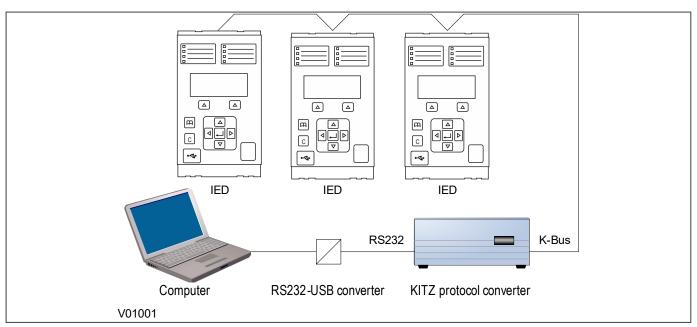
Figure 378: Remote communication using K-Bus
