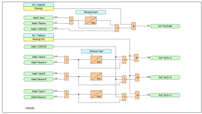
Figure 130: Aided Scheme Blocking 2 Tripping logic
