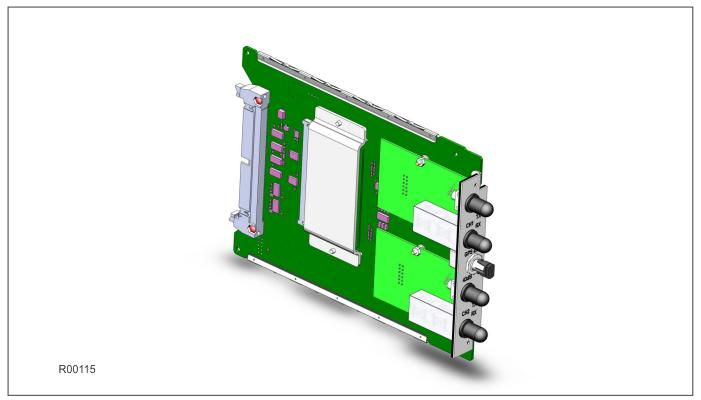
Figure 32: Fully populated Coprocessor board
