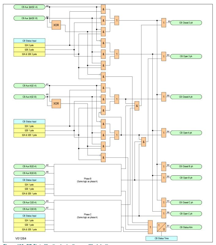
Figure 186: CB State Monitor logic diagram (Module 1)
