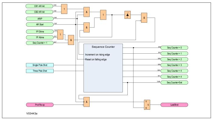
Figure 239: Autoreclose Sequence Counter logic diagram (Module 18)
