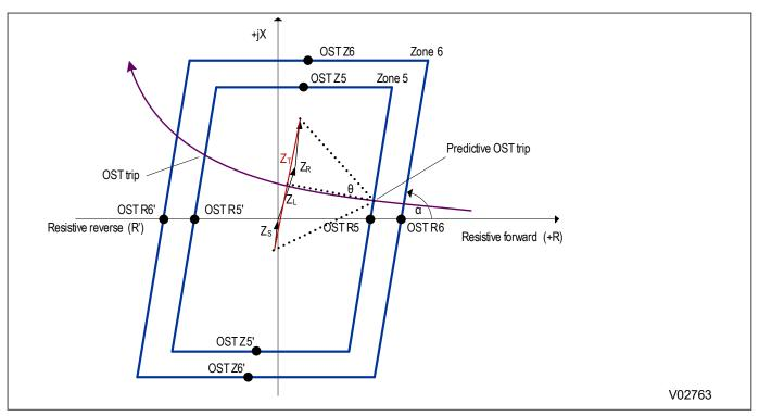
Figure 177: Setting determination for the positive sequence resistive component R5
