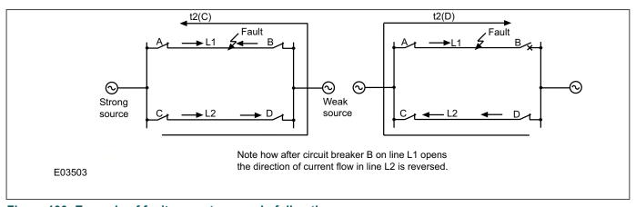
Figure 100: Example of fault current reversal of direction
