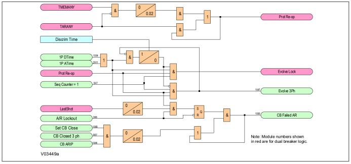
Figure 196: Protection Reoperation and Evolving Fault logic diagram (Module 20)
