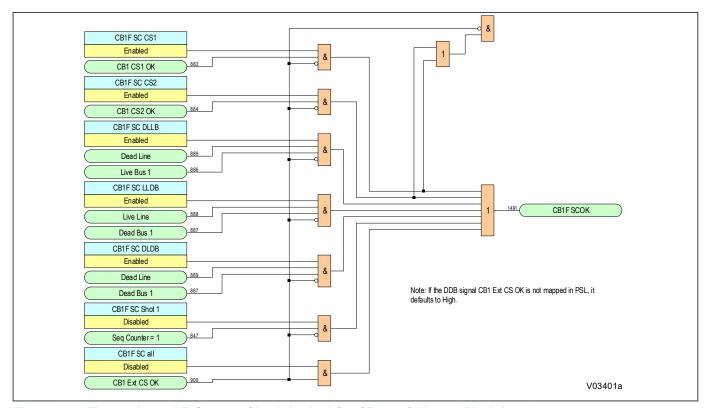
Figure 268: Three-phase AR System Check logic d for CB1 as follower (Module 47)
