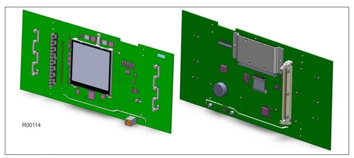
Figure 14: Main processor board
