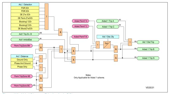
Figure 108: Aided Distance Tripping logic BCh
