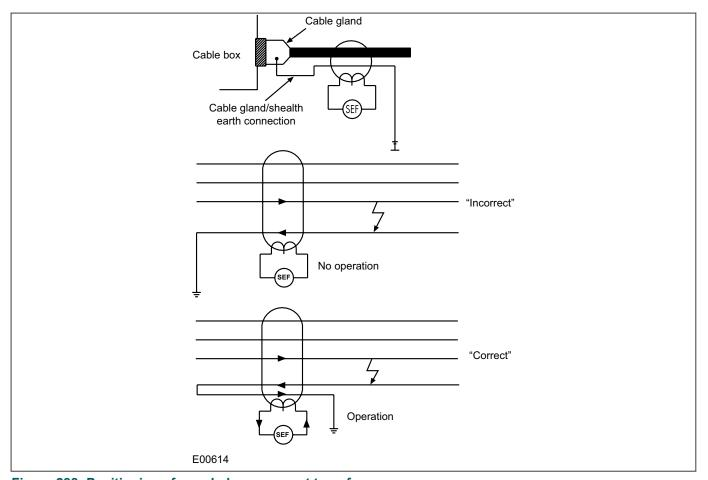
Figure 288: Positioning of core balance current transformers
