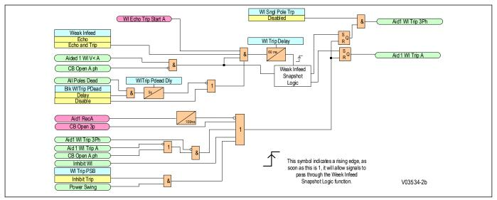
Figure 114: POR Aided Tripping logic ACh (2 of 2) – Weak Infeed Trip
