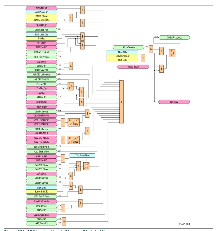
Figure 259: CB2 Lockout Logic Diagram (Module 56)
