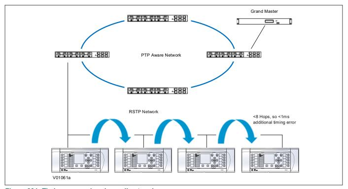
Figure 391: Timing error using ring or line topology
