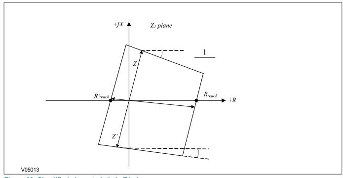
Figure 63: Simplified characteristic in Z1 plane
