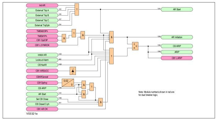
Figure 198: Autoreclose In Progress logic diagram (Module 16)
