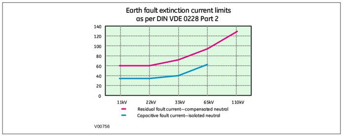
Figure 78: Current level (amps) at which transient faults are self-extinguishing
