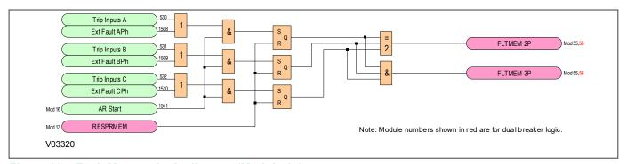
Figure 197: Fault Memory logic diagram (Module 15)
