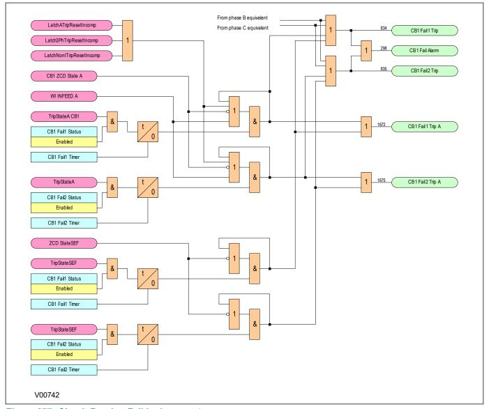
Figure 277: Circuit Breaker Fail logic - part 4
