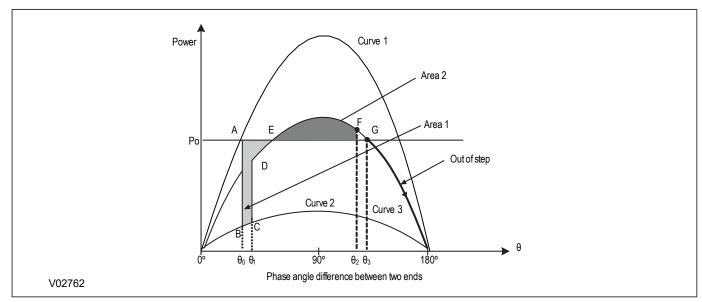
Figure 176: Power transfer in relation to angle difference θ between 2 ends
