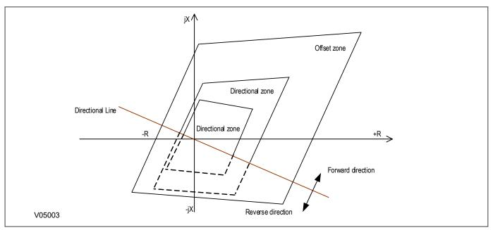
Figure 56: Quadrilateral Characteristic featuring 2 directional forward zones and 1 offset zone
