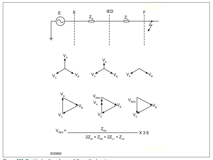
Figure 306: Residual voltage for a solidly earthed system
