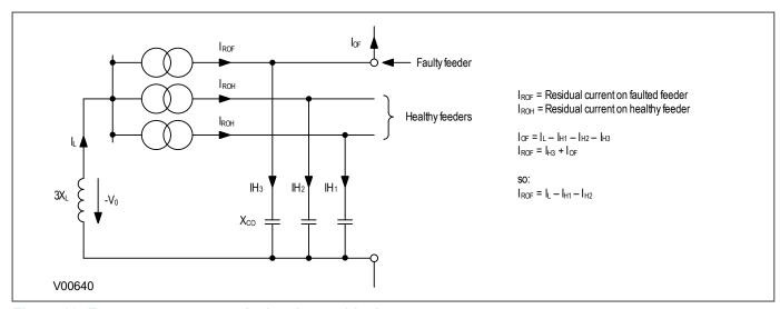
Figure 82: Zero sequence network showing residual currents
