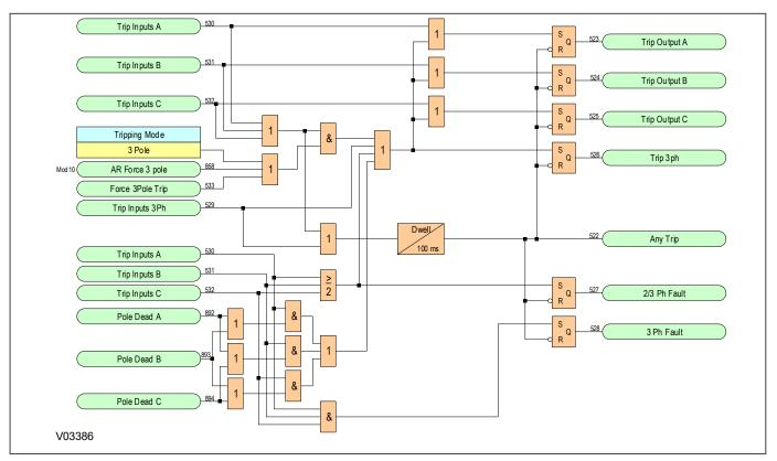
Figure 217: Circuit Breaker Trip Conversion Logic Diagram (Module 63)
