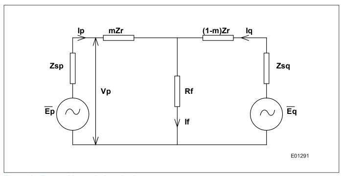
Figure 315: Two machine equivalent circuit
