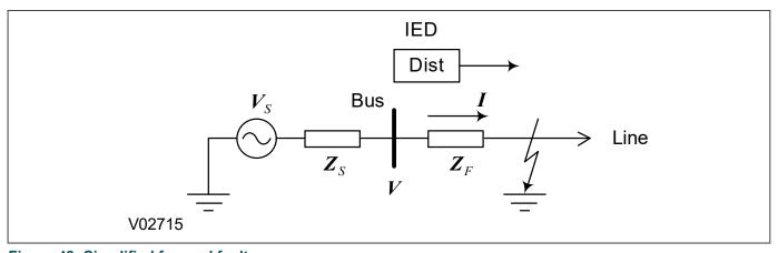
Figure 48: Simplified forward fault
