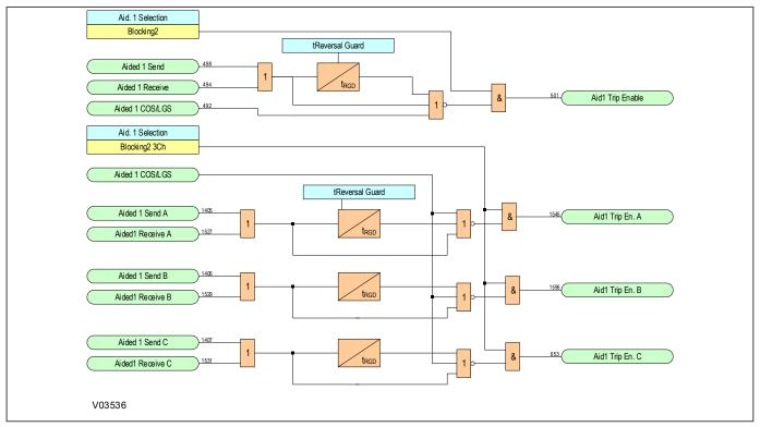
Figure 117: Aided Scheme Blocking 2 Tripping logic
