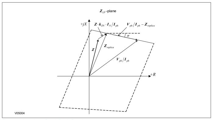
Figure 59: Impedance Reach line in Z<sub>LP</sub> plane
