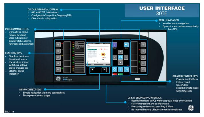
Figure 9: HMI panel
