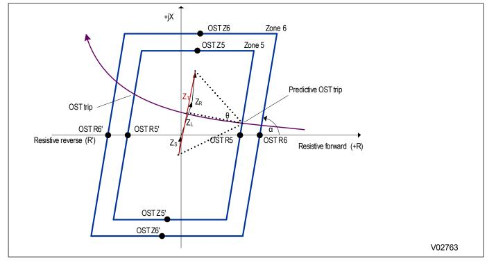
Figure 173: OST setting determination for the positive sequence resistive component OST R5
