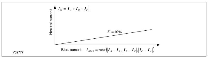
**Figure 85: Biased Neutral Current Detector**
