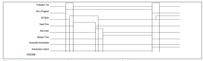
Figure 182: Autoreclose sequence for an evolving or permanent fault
