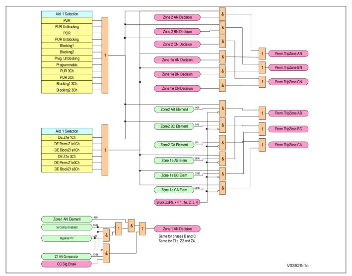
Figure 105: Aided Distance Tripping logic 1Ch (1 of 2)
