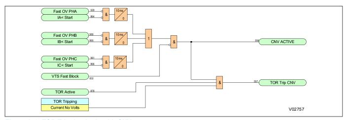
Figure 153: TOR Tripping logic with CNV
