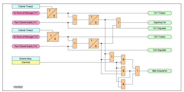
Figure 369: IM64 channel fail and scheme fail logic
