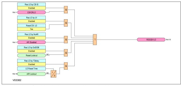
Figure 332: Reset Circuit Breaker Lockout Logic Diagram (Module 57)
