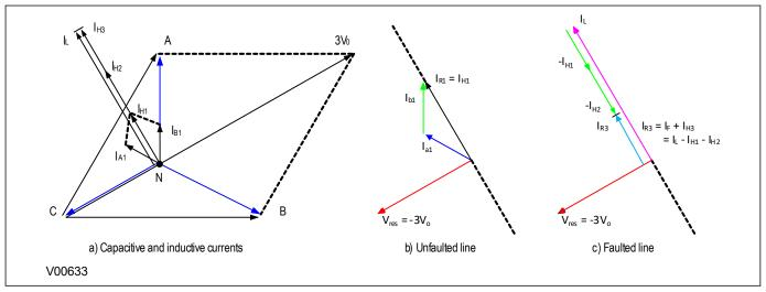
Figure 81: Phasors for a phase C earth fault in a Petersen Coil earthed system
