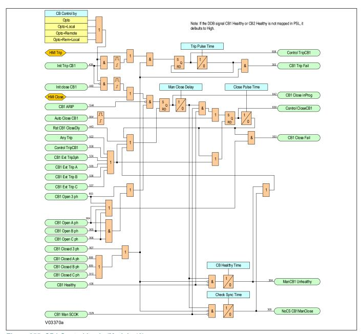
Figure 255: CB1 Control Logic (Module 43)
