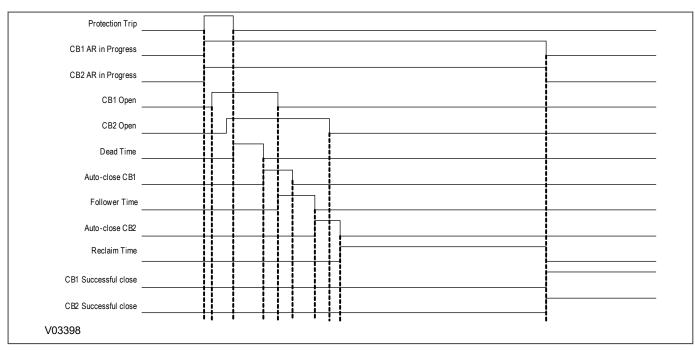
Figure 181: Dual CB Autoreclose Sequence for a Transient Fault
