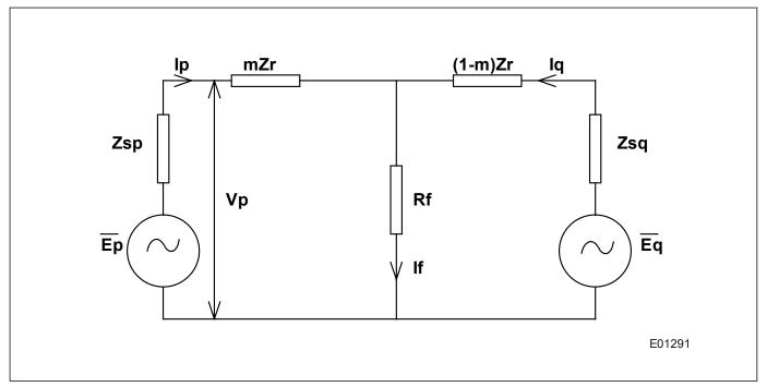
Figure 317: Two machine equivalent circuit
