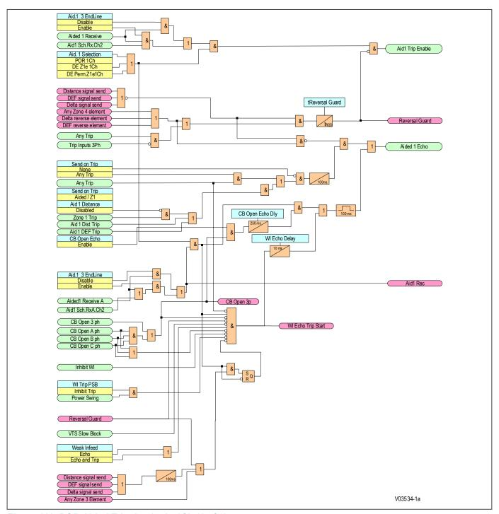
Figure 111: POR Aided Tripping logic 1Ch (1 of 2)
