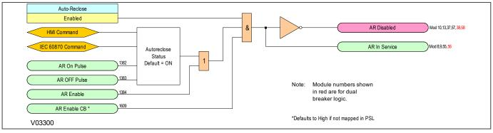
Figure 190: Autoreclose Enable logic diagram (Module 5)
