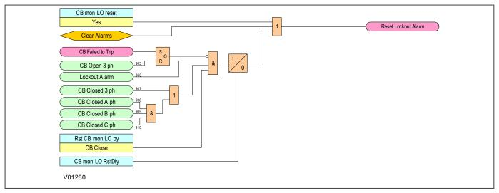
Figure 327: Reset Lockout Alarm logic diagram
