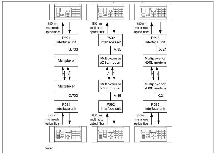
Figure 368: Interfacing to PCM multiplexers
