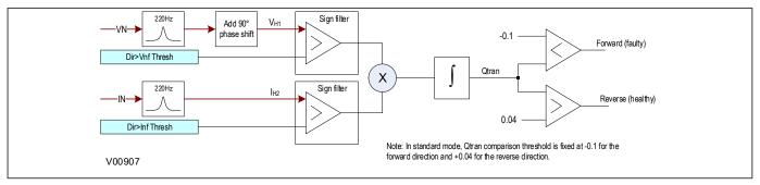
Figure 299: Direction Detector Logic - Standard Mode
