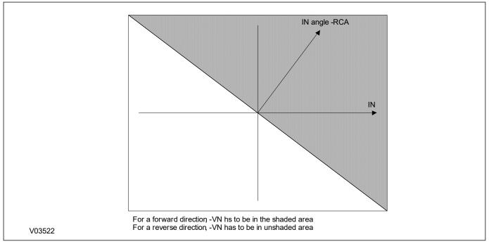
**Figure 118: Virtual Current Polarization**
