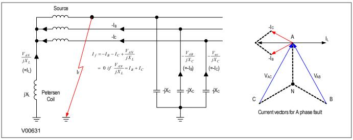
Figure 79: Earth fault in Petersen Coil earthed system
