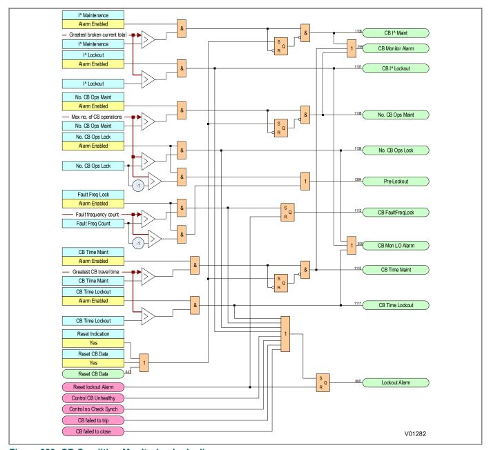
Figure 329: CB Condition Monitoring logic diagram
