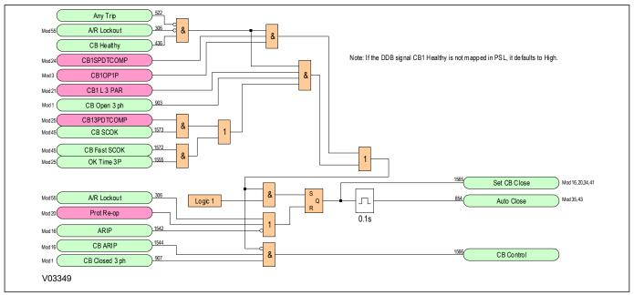
Figure 205: Circuit Breaker Autoclose Logic Diagram (Module 32)
