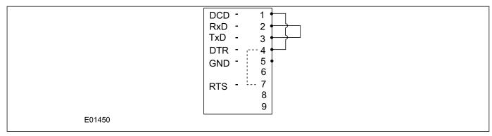
Figure 400: InterMicom loopback testing
