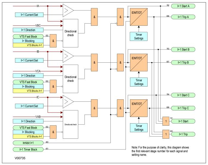
Figure 279: Phase Overcurrent Protection logic diagram
