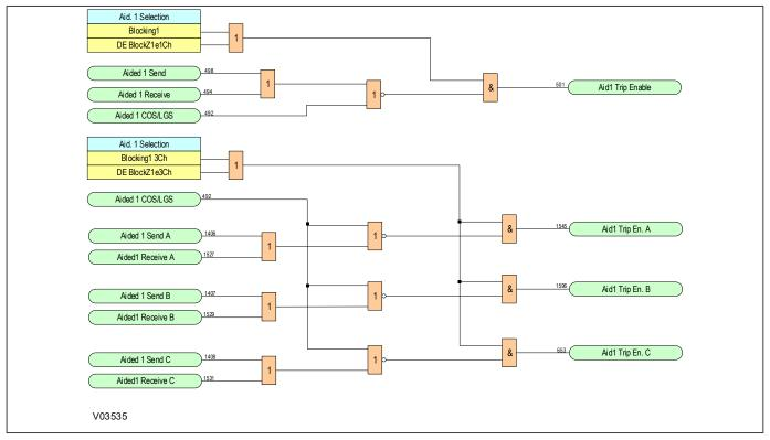
Figure 139: Aided Scheme Blocking 1 Tripping logic
