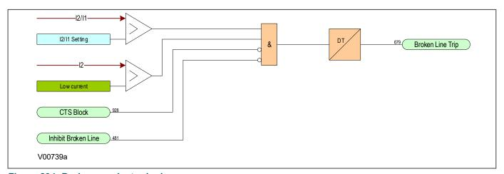
Figure 294: Broken conductor logic
