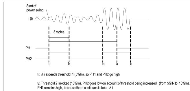
$t_3$ : Fault inception .  $\Delta$  i exceeds threshold 2 (10%ln), so PH2 goes high
