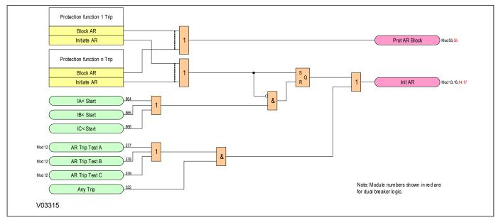
Figure 193: Autoreclose Initiation logic diagram (Module 11)
