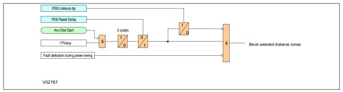
Figure 163: Power swing blocking Logic
