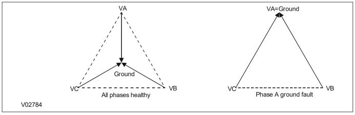
Figure 84: Voltage distribution in an isolated system for a Phase-A-to-Earth fault
