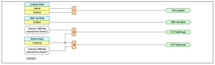
Figure 370: IM64 general alarm signals logic
