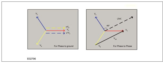
Figure 52: Cross polarizing voltage for phase to ground and phase to phase faults
