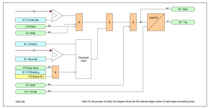
Figure 281: Negative Phase Sequence Overcurrent Protection logic diagram
