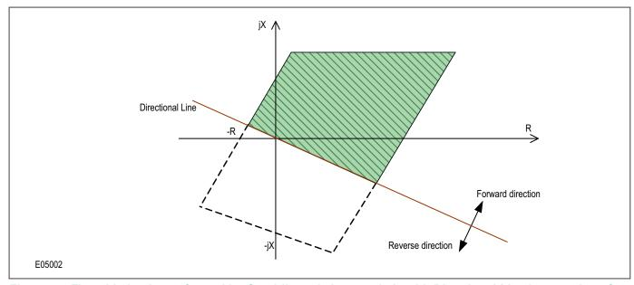
Figure 57: Five-sided polygon formed by Quadrilateral characteristic with Directional-Line intersection of Reverse Impedance Reach Line
