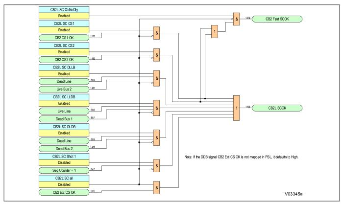
Figure 267: Three-phase AR System Check logic diagram for CB2 as leader (Module 46)
