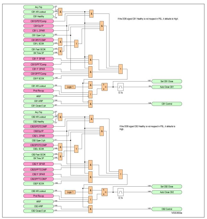
Figure 248: Circuit Breaker Autoclose Logic Diagram (Modules 32 & 33)
