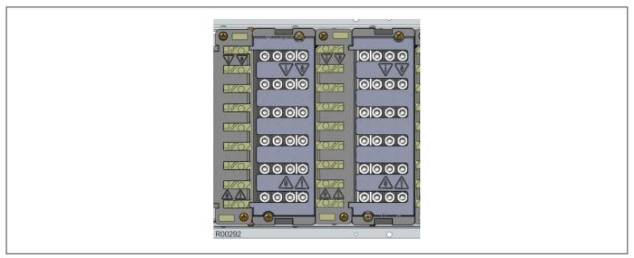
Figure 12: Example - fitted IP2x shields (cabling omitted for clarity)
