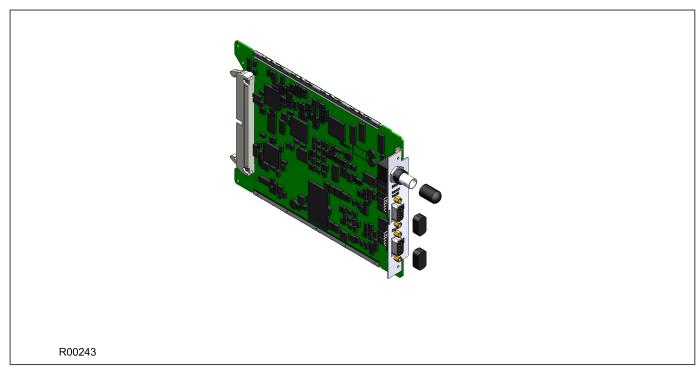
Figure 29: Rear communication board
