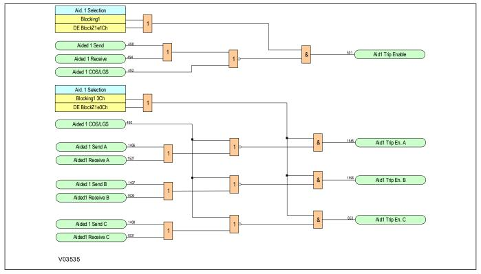
Figure 116: Aided Scheme Blocking 1 Tripping logic
