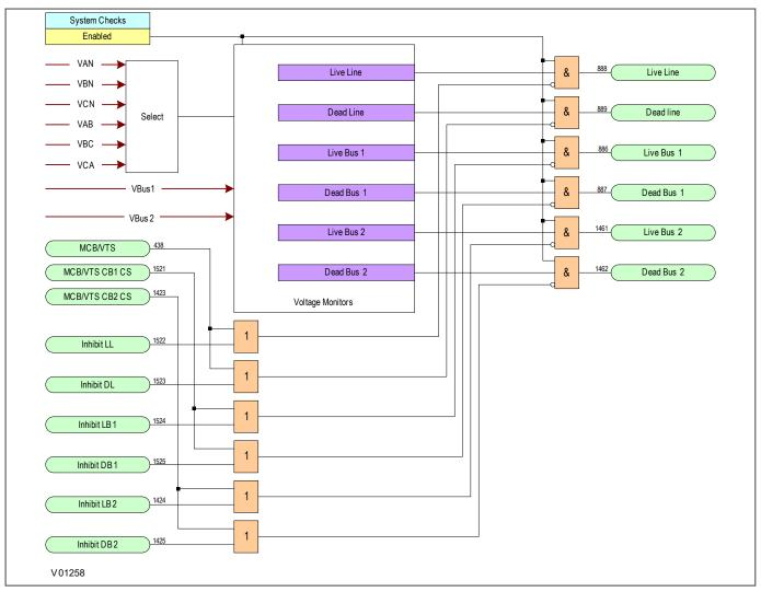
Figure 346: Voltage Monitor for CB Closure (Module 59)
