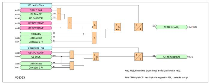
Figure 210: Circuit Breaker Healthy and System Check Timers Healthy logic diagram (Module 39)
