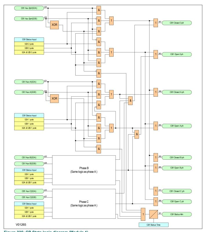
Figure 335: CB State logic diagram (Module 1)
