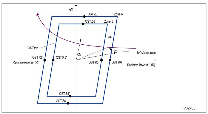
Figure 175: Example of timer reset due to MOVs operation
