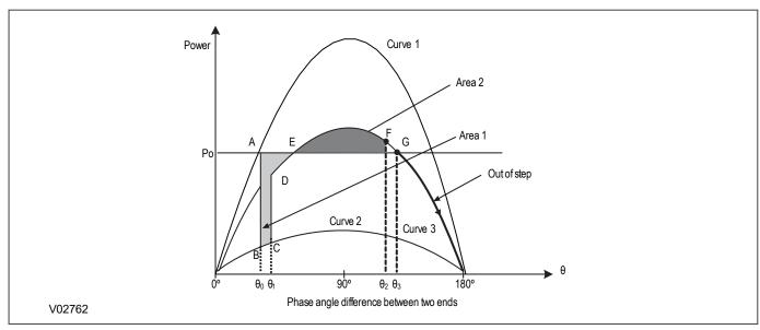
Figure 158: Power transfer related to angular difference between two generation sources
