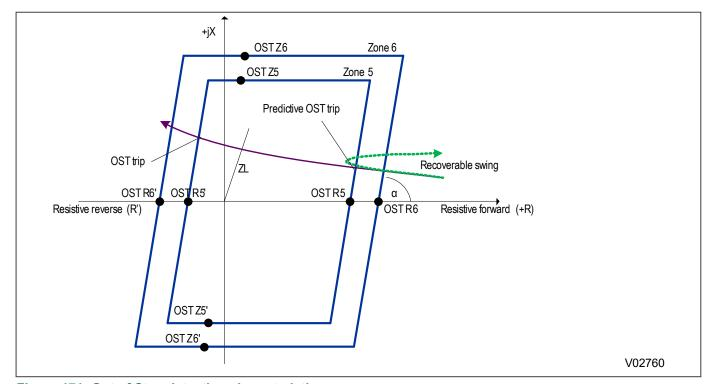
Figure 171: Out of Step detection characteristic
