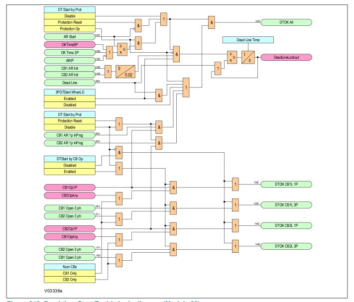
Figure 242: Dead time Start Enable logic diagram (Module 22)
