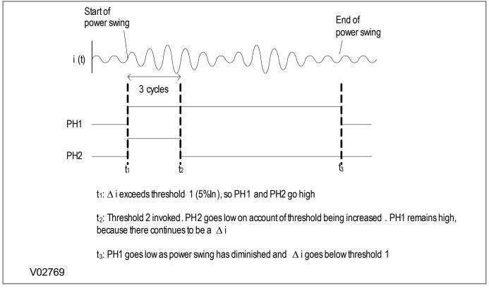
Figure 159: Phase selector timing for power swing condition
