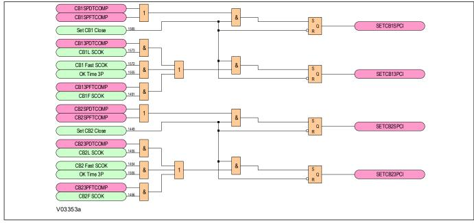
Figure 249: Prepare Reclaim Initiation logic diagram (Module 34)
