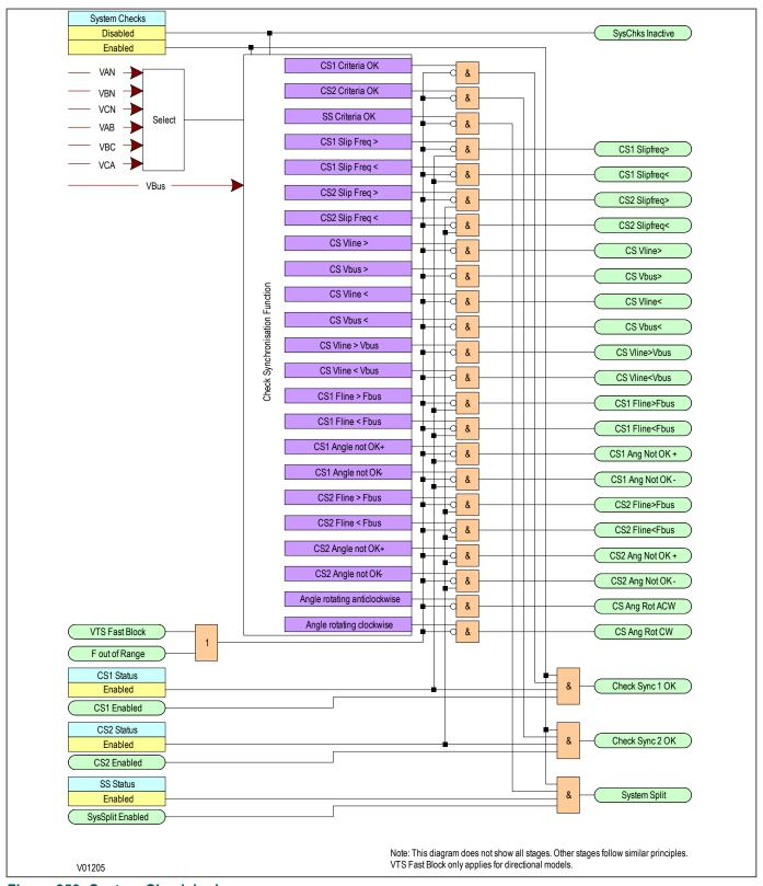
Figure 350: System Check logic
