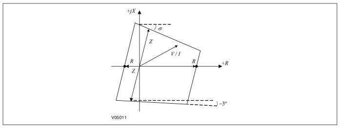
Figure 72: Phase Fault Quadrilateral characteristic summary
