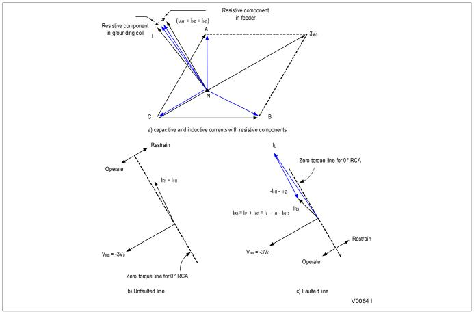
Figure 83: Phase C earth fault in Petersen Coil earthed system: practical case with resistance present
