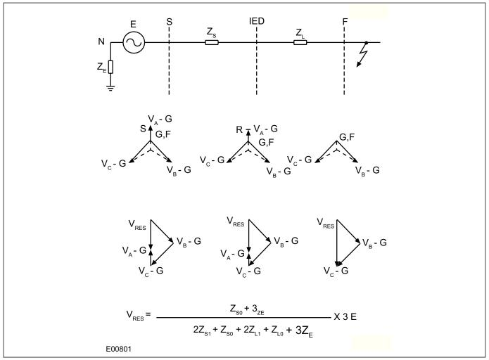
Figure 307: Residual voltage for an impedance earthed system
