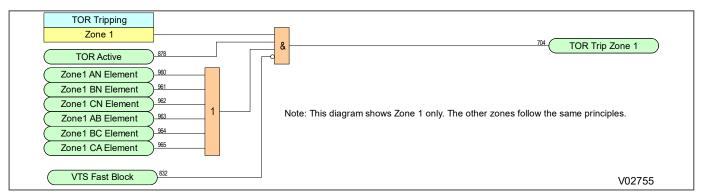
Figure 152: TOR Tripping logic for appropriate zones
