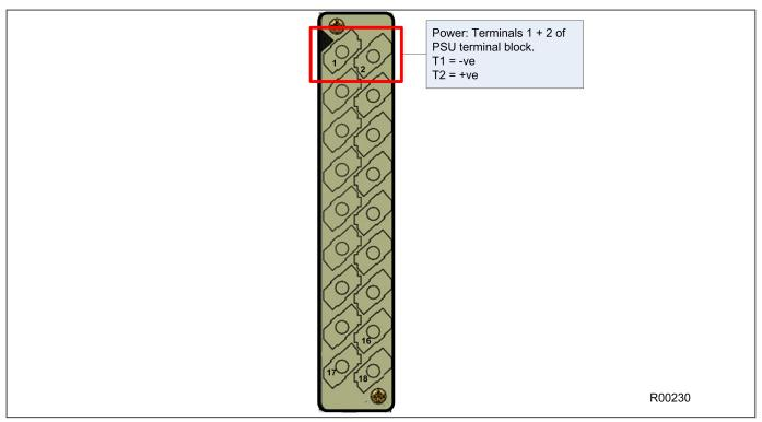
Figure 17: Power supply terminals
