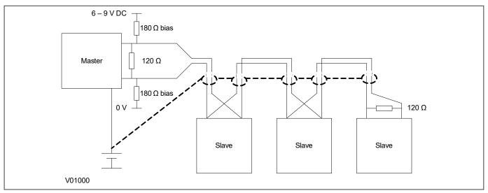
Figure 377: RS485 biasing circuit
