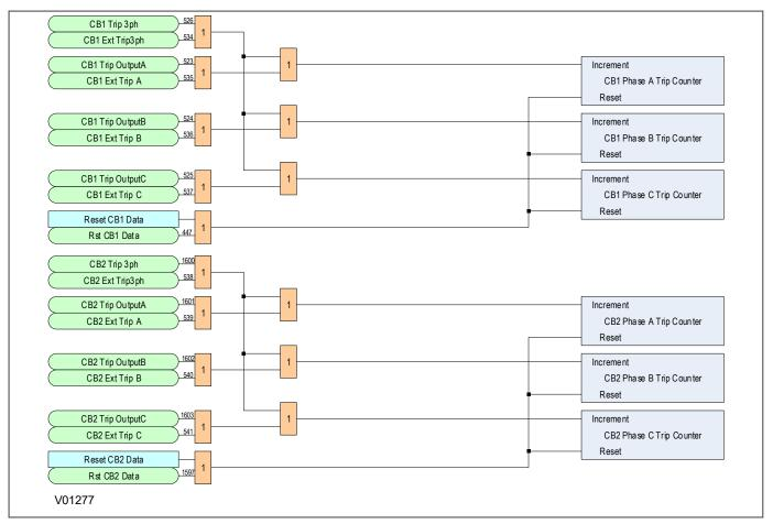
Figure 322: CB Trip Counter logic diagram
