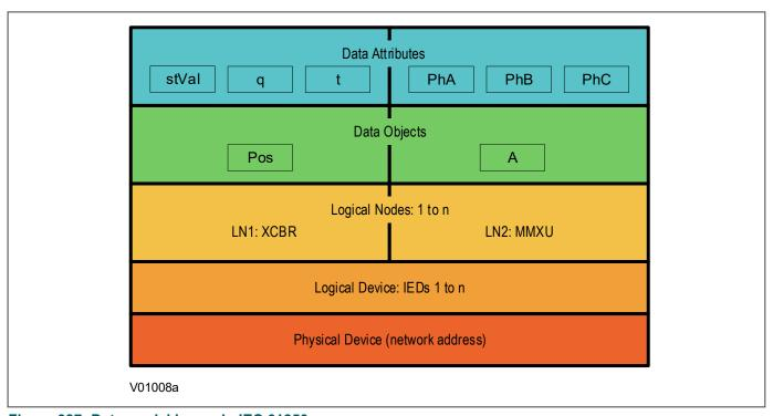
Figure 387: Data model layers in IEC 61850
