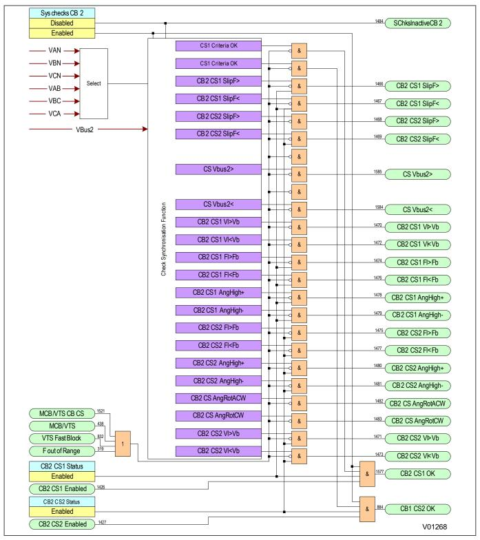
Figure 349: Check Synchronisation Monitor for CB2 closure (Module 61)
