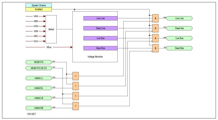
Figure 345: Voltage Monitor for CB Closure (Module 59)
