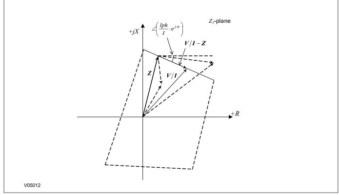
Figure 58: Impedance Reach line in Z1 plane
