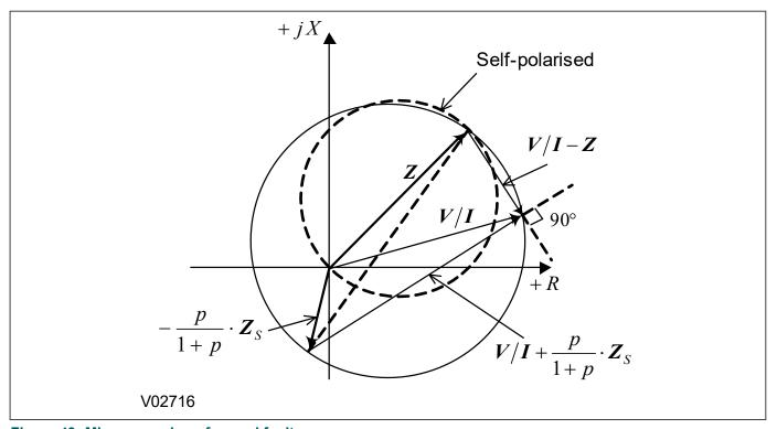
Figure 49: Mho expansion - forward fault
