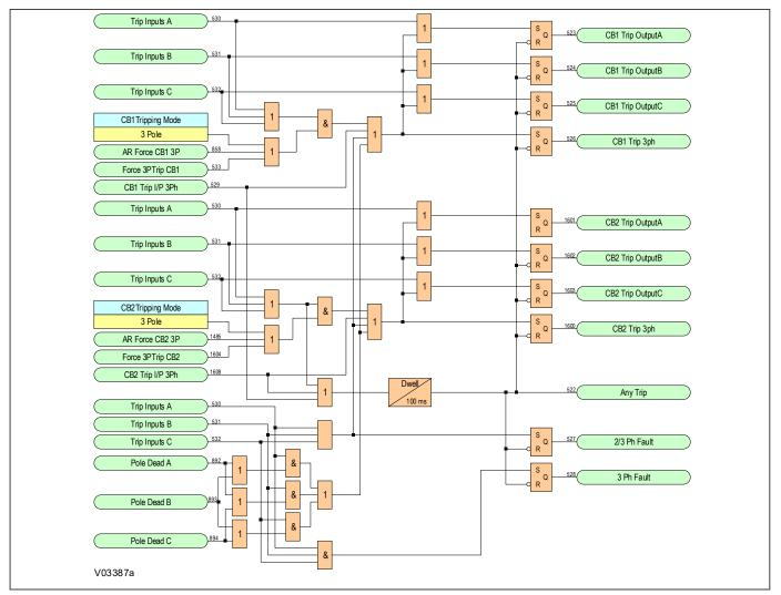
Figure 262: Circuit Breaker Trip Conversion Logic Diagram (Module 63)
