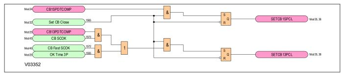
Figure 206: Prepare Reclaim Initiation Logic Diagram (Module 34)
