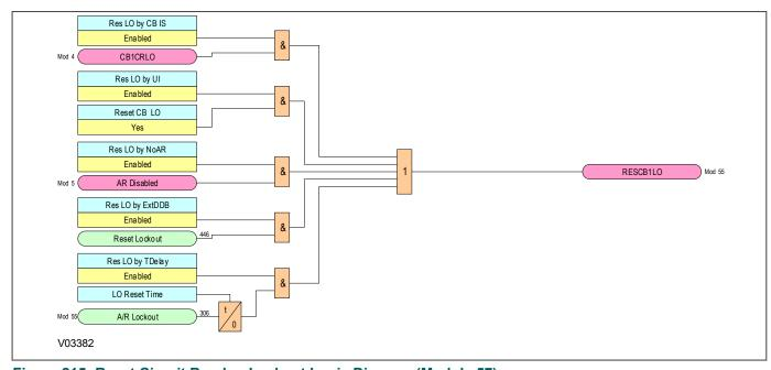
Figure 215: Reset Circuit Breaker Lockout Logic Diagram (Module 57)
