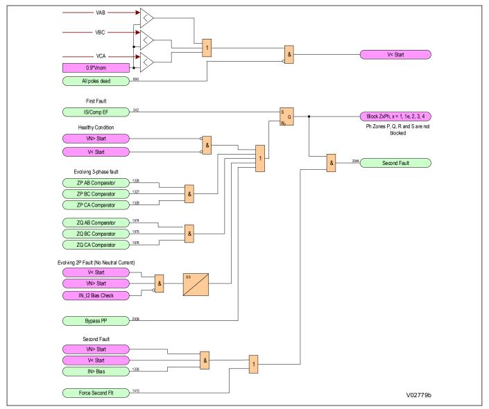
Figure 87: Second earth fault detection logic
