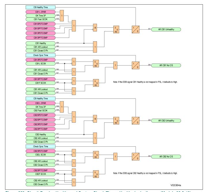
Figure 253: Circuit Breaker Healthy and System Check Timers Healthy logic diagram (Module 38 & 40)
