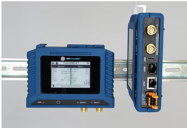
Figure 2-6. DIN Rail Attachment examples (Pull down tab to release from rail)
