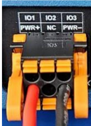
Figure 2-3. 6-pin Power & I/O Connector (P/N 73-1194A85)
