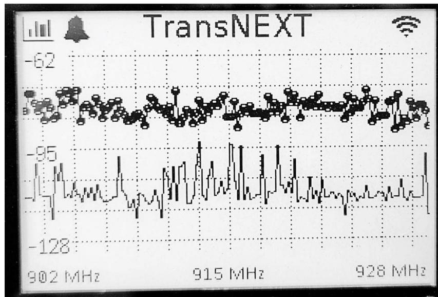
**NOTE** The Spectrum Analyzer Page is intended as a simple tool to detect easily identified blockers in the FHSS band. It is based on a simple collection of signal strength and only operates over the bands in which the radio operates. For advanced troubleshooting use of RF test equipment is still recommended.
