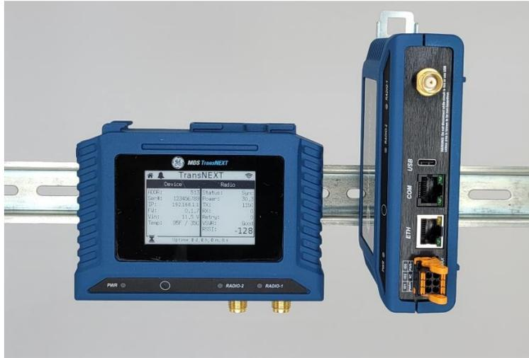
**Figure 2-7. DIN Rail Attachment examples**
