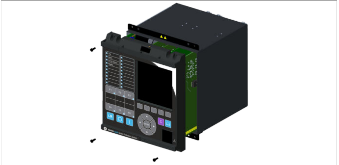
Figure 6: Exploded view of IED - 30TE IEC version
