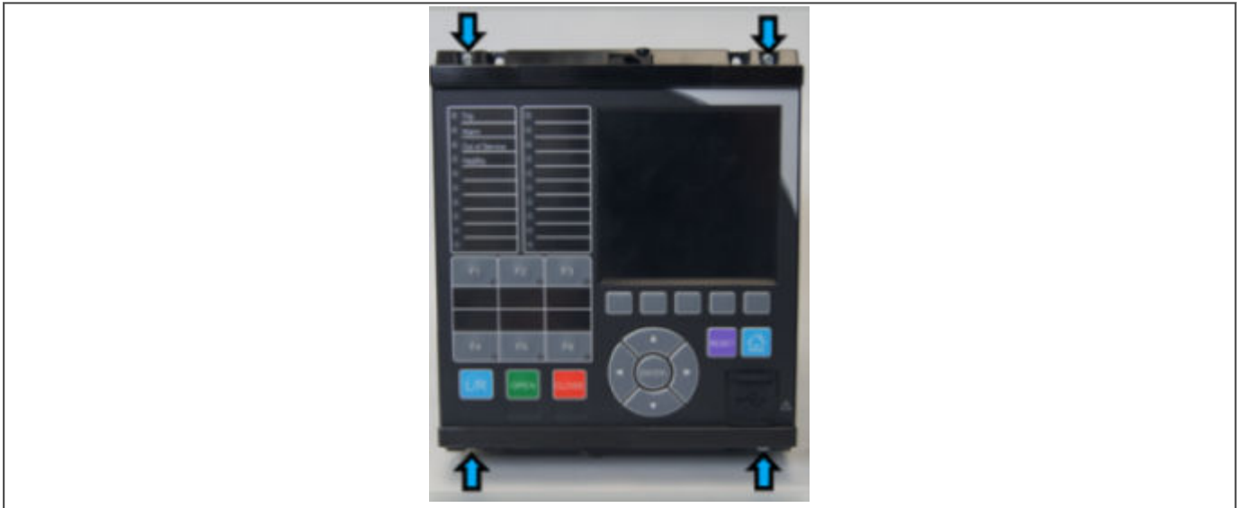
Figure 189: 30TE (without cam) screws placement
