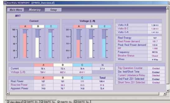
Monitor breaker equipment with predefined screens.
