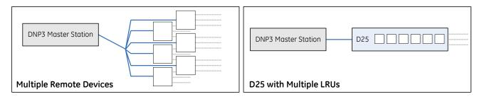
**Protocol Conversion.** With a suite of over 120 protocols, including IEC 61850, Modbus®, DNP, SPABus, Courier, and IEC 101/103/104; the D25 can translate multiple protocols over multiple channels. This is often useful in retrofit situations.
