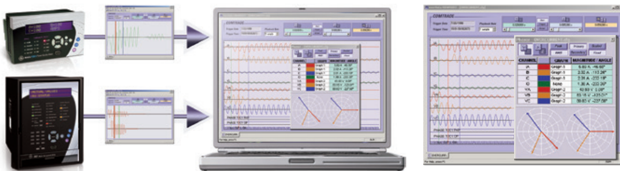
View and analyze waveform fault data retrieved from devices.
