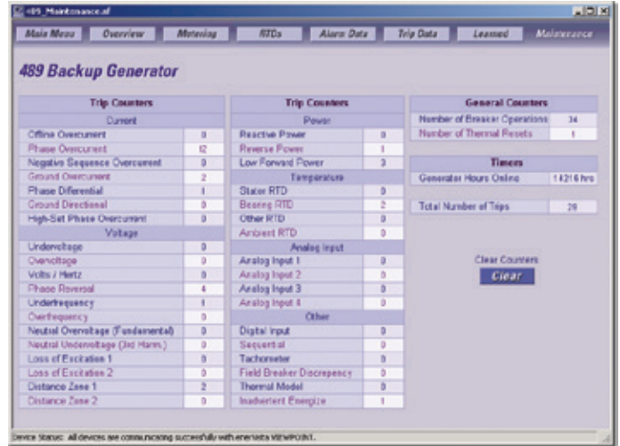
Improve maintenance efficiency by analyzing trip operations.
