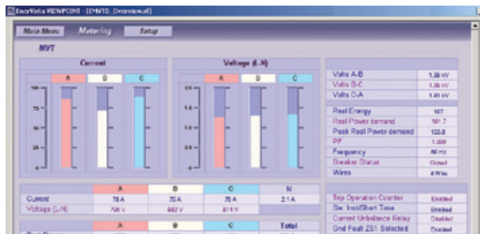
Monitor breaker equipment with predefined screens.
