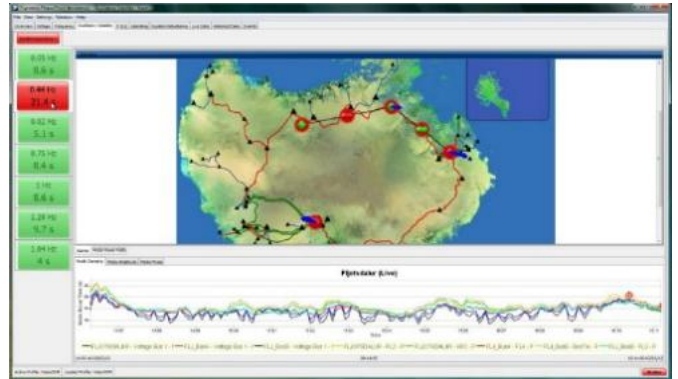
Figure 4 PhasorPoint oscillatory stability management (OSM)
